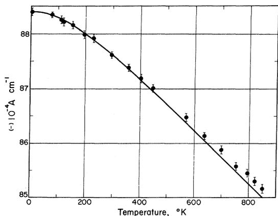
FIG. 3. Temperature dependence of the hyperfine-coupling parameter  $A$ . The points are experimental, while the solid curve is the explicit temperature dependence after correcting for thermal expansion.
