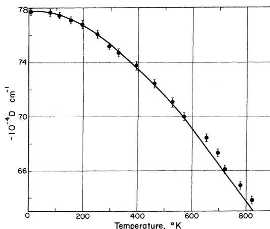
FIG. 1. Temperature dependence of the axial crystalline-field parameter  $D$ . The points are experimental, while the solid curve is the explicit temperature dependence after correcting for thermal expansion.
