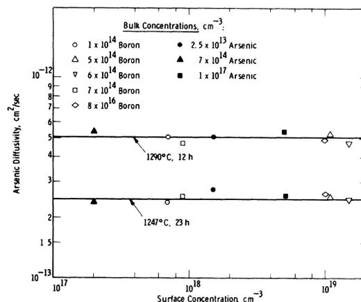
FIG. 7. Concentration dependence of arsenic diffusivity in (111) silicon.
