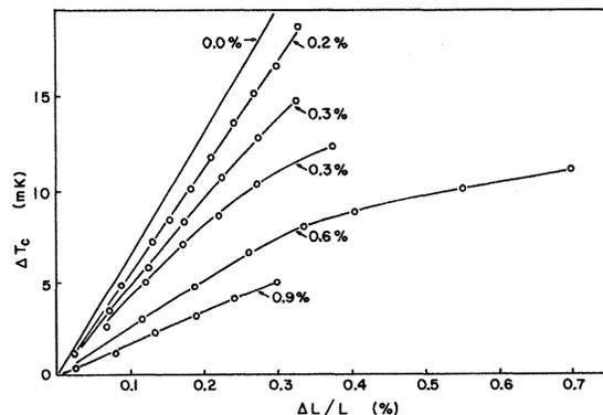
FIG. 3. Shift in transition temperature  $T_c$  as a function of strain for Cd content up to 0.9 at.%. The transition temperature was taken to be the midpoint of the resistive transition. The two curves at 0.3 at.% represent the uncertainty in puller calibration and alloy content. One can see the change in initial slope and the departure from linearity of these curves as the Cd content is increased.
