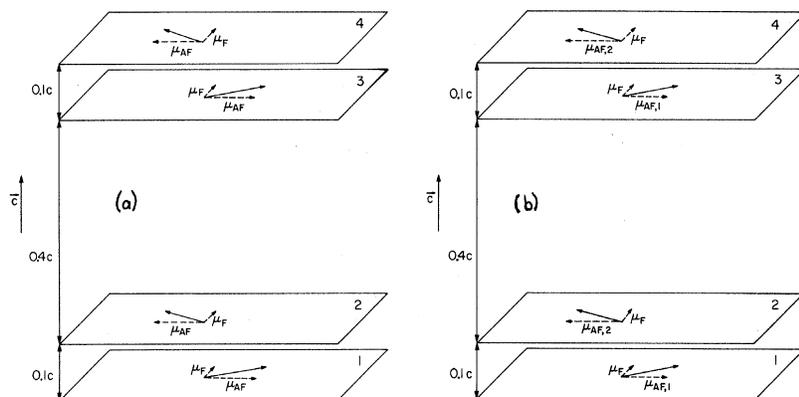
FIG. 2. Basis of the spiral structure: The planes indicate layers of atoms with the same phase.  $c$  is the dimension of the chemical cell along the  $c$  axis. The actual magnetic structure is obtained by rotating the moments on each layer of an angle proportional to the distance from the bottom layer. (a) Basis for model 1: all magnetic moments are equal. (b) Basis for model 2: two sets of magnetic moments.
