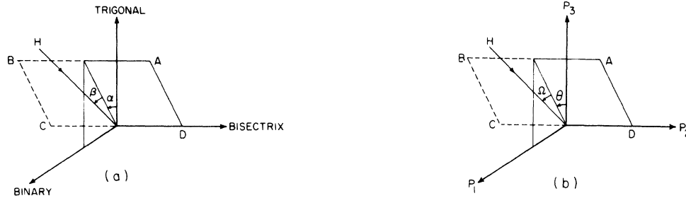
FIG. 3. Definition of magnetic field direction in (a) crystallographic-axis system and (b) ellipsoid principal-axis system. In both cases plane ABCD is rotated counter clockwise about the bisectrix or p_2 axis as one looks along it in the negative direction. \beta and \Omega are angles in these rotated planes. The rotation about the bisectrix or p_2 axis is specified as occurring first.
