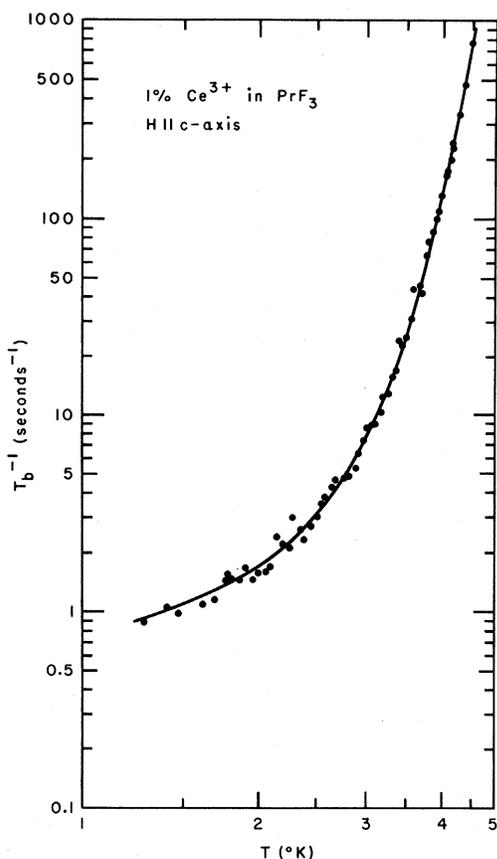
FIG. 3. Spin-lattice data for 1%  $\text{Ce}^{3+}$  in  $\text{PrF}_3$  are fitted by  $T_b^{-1} = 0.753T + 0.276 \times 10^{-3}T^9 + 0.171 \times 10^{11}e^{-78.3/T}$  for  $H$  parallel to the  $c$  axis.
