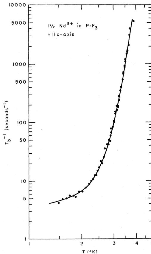
FIG. 1. Spin-lattice data for 1%  $Nd^{3+}$  in  $PrF_3$  are fitted by  $T_b^{-1} = 2.85T + 0.214 \times 10^{-2} T^9 + 0.378 \times 10^{11} e^{-61.5/T}$  for  $H$  parallel to the  $c$  axis.
