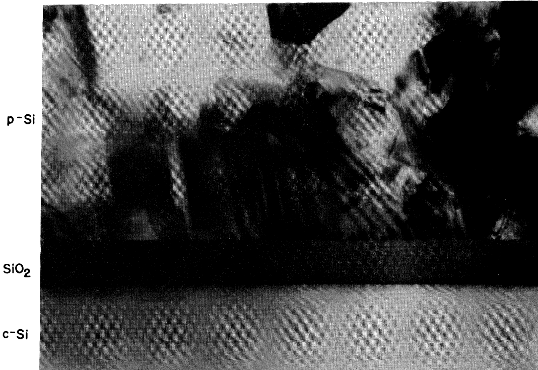
FIG. 2. Micrograph of the cross section of the heavily doped large-grain polycrystalline film used to obtain the data of Fig. 1. The 1000-Å thermal oxide and single-crystal Si substrate are the dark and light gray regions, respectively.
