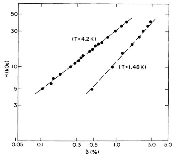
FIG. 3. Positive MR as a function of field for a Nb film with  $R_{\square} = 11.8$  k $\Omega$  (at 4.2 K) measured at 4.2 and 1.48 K (field perpendicular to film surface).
