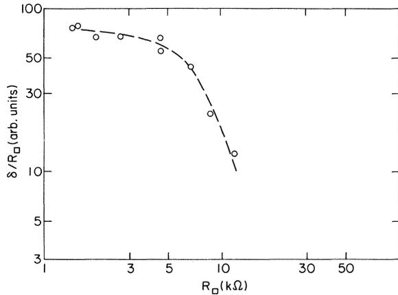
FIG. 4. Magnitude of the MR at 4.2 K and 7 kOe vs sheet resistance.
