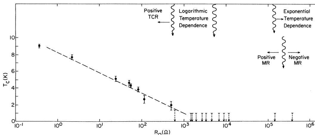
FIG. 1. Superconducting transition temperature  $T_c$  of the Nb films is plotted as a function of the sheet resistance at 4.2 K (the values of  $R_{\square}$  where electrical resistance measurements were made and no  $T_c$  were found are indicated by arrows). Also included are the ranges in terms of  $R_{\square}$  where qualitative change in the transport properties were observed.
