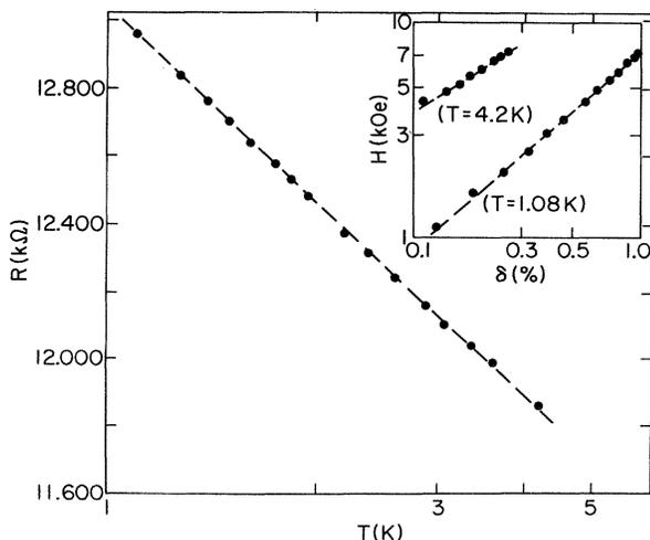
FIG. 2. Resistance vs temperature for a Nb film with  $R_{\square} = 4.56$  k $\Omega$  (at 4.2 K). Inset shows positive MR for the same Nb film at 4.2 and 1.08 K (field perpendicular to the film's plane).
