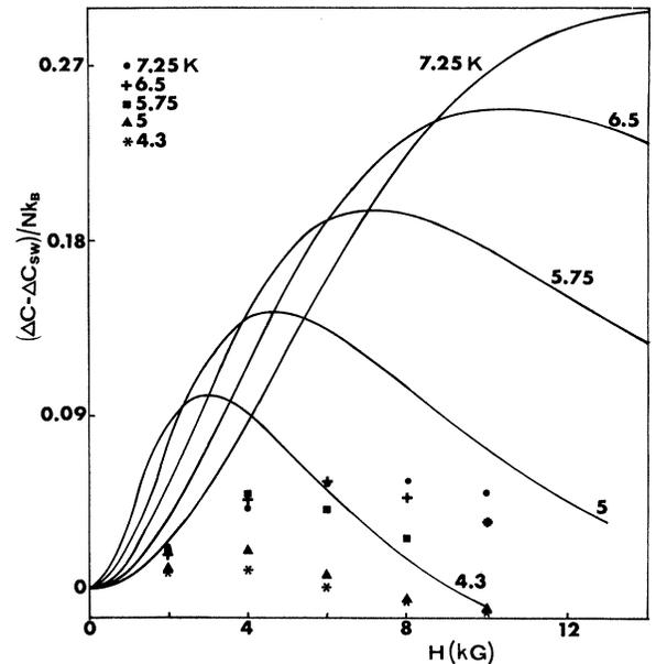
FIG. 3. Field dependence of  $(\Delta C - \Delta C_{sw}) / Nk_B$  at different values of  $T$ . Full line: TM data. Symbols: experimental data (Ref. 4) for CsNiF<sub>3</sub>.
