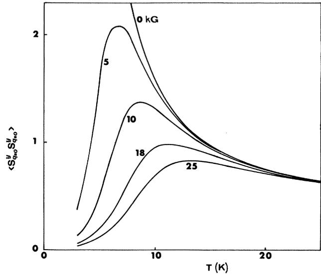
FIG. 5. TM data for the temperature dependence of  $S^{\parallel}(q=0)$  at different fields.
