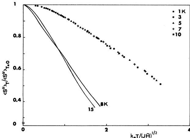
FIG. 1. Universal plot for reduced magnetization  $\langle S^y \rangle_T / \langle S^y \rangle_{T=0}$  vs  $k_B T / (\tilde{H}J)^{1/2}$ . Curves: TM data. Symbols: quantum LSW theory results.
