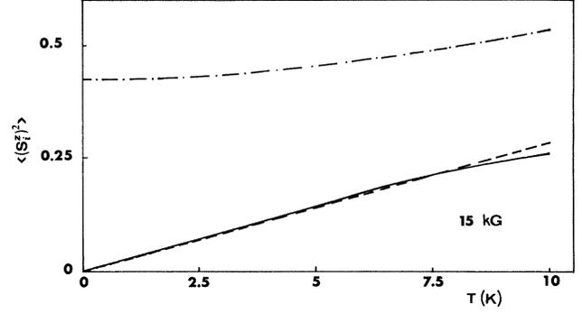
FIG. 2. Temperature dependence of the out-of-plane fluctuations  $\langle (S_f^z)^2 \rangle$  for  $H = 15$  kG. Full line: TM data. Dashed line: classical LSW results. Dashed-dotted line: quantum LSW results.
