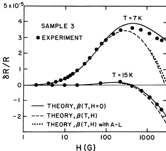
FIG. 1. Normalized magnetoresistance for sample 3. Fitting parameters are  $H_{so} = 30$  G, and  $H_i = 3.8$  G at 7 K and 33 G at 15 K. At 15 K, the Aslamasov-Larkin contribution to  $\delta R$  is negligible.
