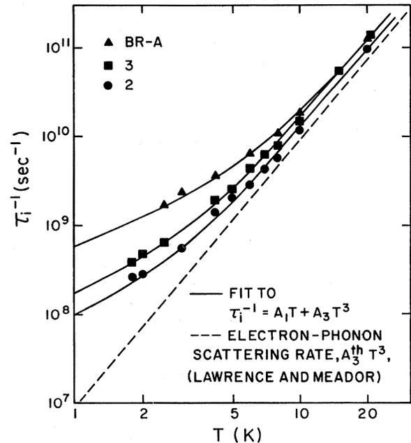
FIG. 2. Inelastic-scattering rate vs temperature. Rate for curve BR-A is from our analysis of magnetoresistance data of sample A, Ref. 6. Values of  $A_1$  and  $A_3$  are listed in Table I. Theoretical electron-phonon scattering rate, Ref. 11, is  $\tau_{ep}^{-1} = 0.91 \times 10^7 T^3$ .
