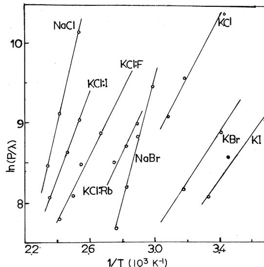
FIG. 4. Arrhenius plots for various powders.  $\ln p/\lambda$  vs  $1/T$  is plotted, where  $\lambda$  is the rate constant,  $p$  is an arbitrary constant, and  $T$  is the temperature (K) at which the decay is recorded. Slopes of the straight lines equal  $E/k$ .
