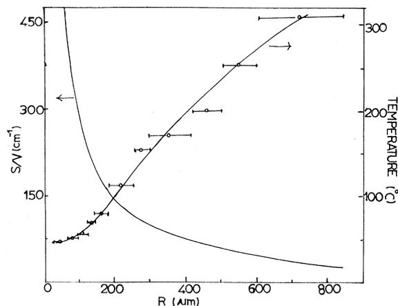
FIG. 10. Stability of coloration as a function of particle size. Temperature required to induce 50% decay in 1 h is taken as a criterion for stability.  $S/V$  ratio ( $3/R$ ) is also plotted.
