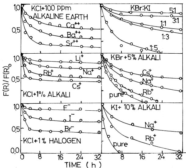
FIG. 5. Inhibition of decay by impurities. Isothermal decay of  $F$  centers in various powders at RT (after Ref. 5).
