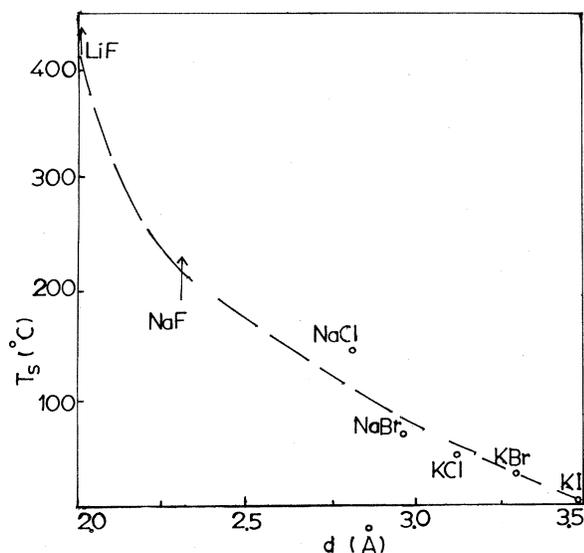
FIG. 3. Stability of coloration of microcrystalline powders of various alkali halides. Temperature  $T_s$  required to induce 50% decay in 2 h in powders 124–140  $\mu\text{m}$  is plotted as a function of nearest-neighbor distance  $d$ . In the case of NaF and LiF, an estimated lower limit of  $T_s$  is shown.
