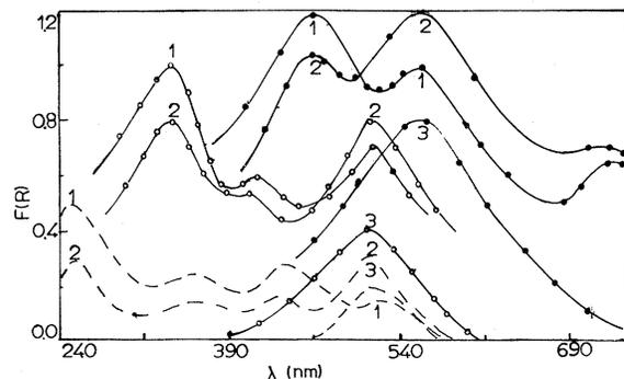
FIG. 2.  $F$ -to-colloid conversion in powders colored in an electrodeless discharge. Dashed curve: LiF—(1) as colored, (2) after 8 h at 400°C, and (3) after 1 h at 400°C; curve through open circles: NaF—(1) as colored, (2) after storing at 175°C for 30 min, and (3) for 1 h; curve through closed circles: NaCl—(1) as colored, (2) after storing at 80°C for 30 min, and (3) for 1 h.
