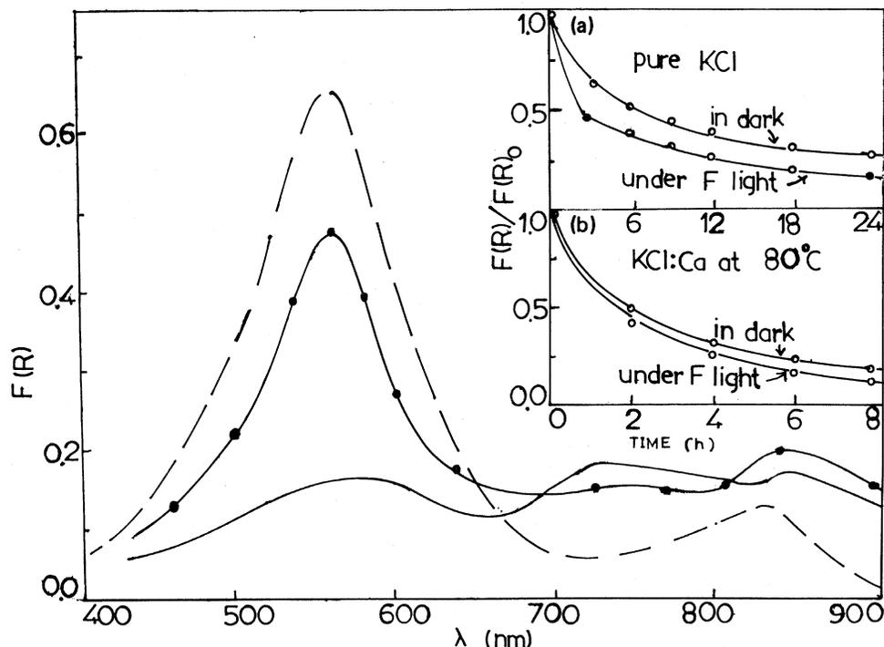
FIG. 8. Effect of optical bleaching on decay. — — —: as-colored KCl powder; — · —: after 15 min  $F$  bleaching; —: after 6 h  $F$  bleaching. Inset (a) shows decay of  $F$  band in KCl powders stored at RT in dark and under  $F$  light. Inset (b) shows similar results for KCl:Ca powders stored at 80°C.
