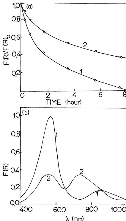
FIG. 11. (a) Isothermal decay of  $F$  centers in microcrystallites: (1) particles ( $600\text{--}850\ \mu\text{m}$ ) obtained by crushing stored at  $300^\circ\text{C}$ ; (2) particles of same size obtained by cleaving stored at  $300^\circ\text{C}$ . (b)  $F$ -colloid conversion in cleaved crystallites. Reflectance spectra of 1, as-colored particles, and 2, after storing at  $300^\circ\text{C}$  for 8 h.
