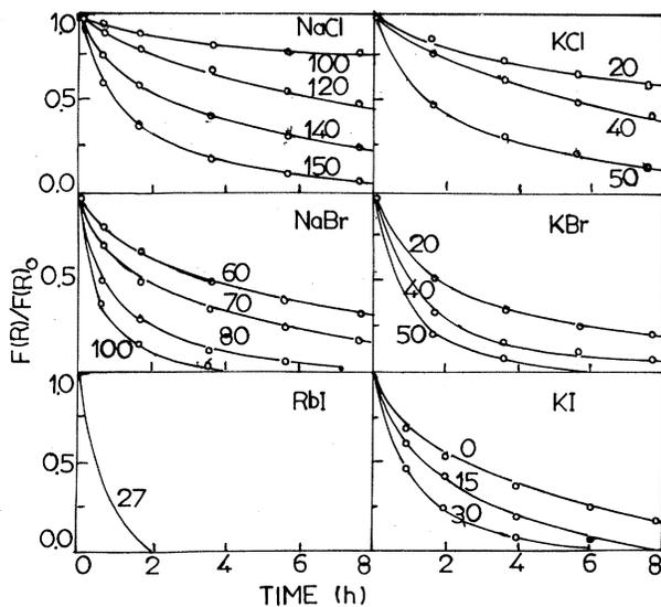
FIG. 1. Isothermal decay of  $F$  centers in microcrystalline powders (124–140  $\mu\text{m}$ ) of various alkali halides at different temperatures (numbers of the curves). The Kubelka-Munk function normalized in terms of initial value at the  $F$ -band maximum is plotted as a function of storage time.
