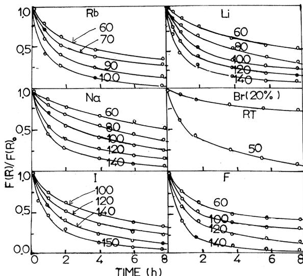
FIG. 6. Isothermal decay of  $F$  centers in KCl powders doped with various impurities (1 mol%) at different temperatures (numbers on curves).
