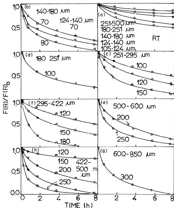
FIG. 9. Effect of particle size on stability of coloration. Isothermal decay of  $F$  centers in powders of varying fineness at different temperatures (numbers on curves) are shown in Figs. (b)–(h). In (a), isothermal decay curves for various particle sizes recorded at RT are plotted. The decay curves for powders in the range 77–105  $\mu\text{m}$  and less than 77  $\mu\text{m}$  are not appreciably slower than shown for 105–124  $\mu\text{m}$ .
