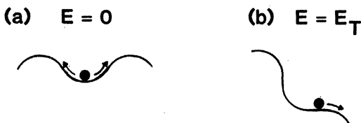
FIG. 1. Classical overdamped oscillator model: (a) at zero applied dc field, and (b) at threshold.
