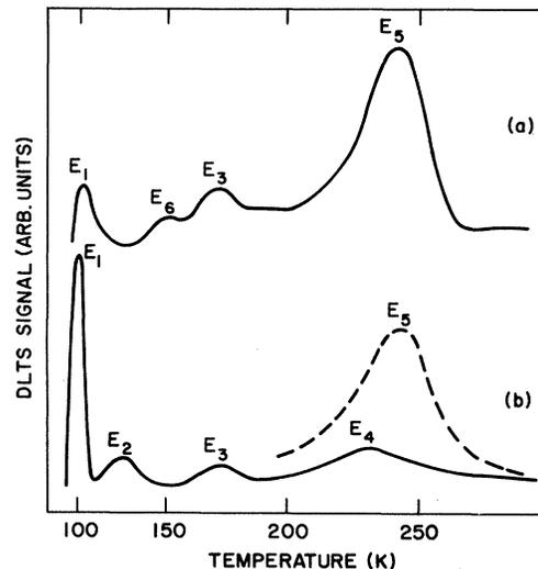
FIG. 1. DLTS spectra of silicon Schottky diodes irradiated with (a) 100-keV and (b) 1-MeV electrons.  $V_B = 2.0 \text{ V}$ .  $V_p = 1.0$  (solid curves) or 1.5 V (dashed curve). The rate window was 8.7 msec.
