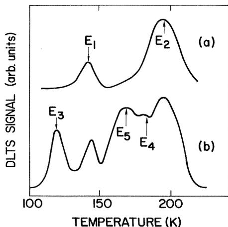
FIG. 2. DLTS spectra for germanium  $p^+$ - $n$  junction diodes irradiated with (a) 540-keV and (b) 2-MeV electrons. The rate window was 6.9 msec.
