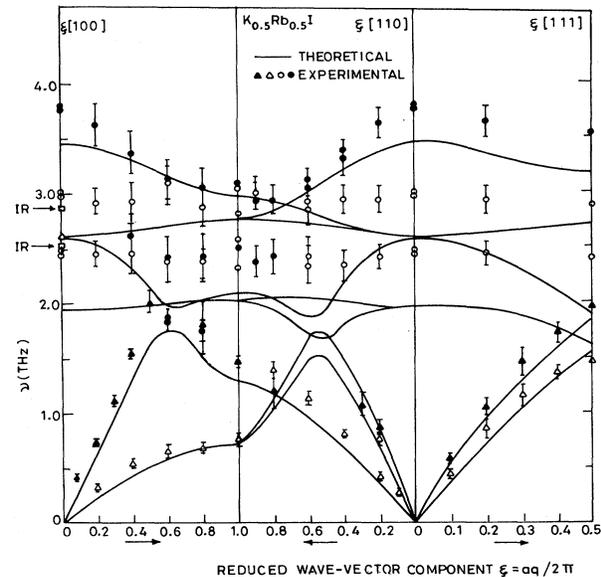
FIG. 1. Phonon dispersion in the mixed crystal  $K_{0.5}Rb_{0.5}I$ . Circles indicate the experimental inelastic neutron scattering (INS) results of Renker *et al.* (Ref. 16); triangles indicate the INS data of Aslam *et al.* (Ref. 14), and squares indicate the infrared (IR) data of Fertel and Perry (Ref. 4).
