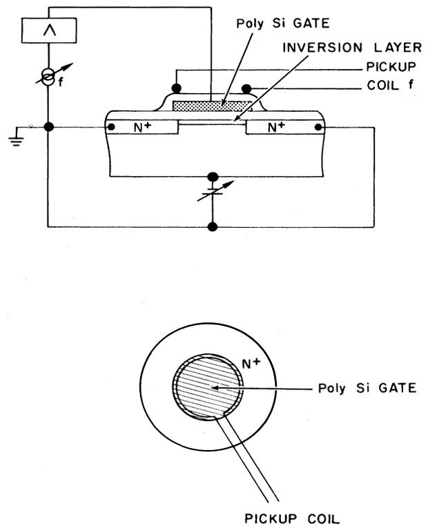
FIG. 2. Schematic diagrams of the sample and measuring configurations.
