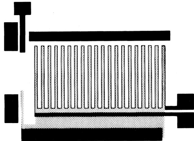
FIG. 3. Gate and pick-up coil geometry of the actual sample. Heavily doped  $n$ -type region surrounds the inversion layer under the gate.
