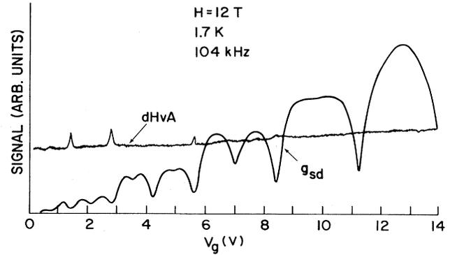
FIG. 5. dHvA detected from the pick-up coil as a function of the gate voltage at  $H=12$  T,  $T=1.7$  K, and modulation frequency at 104 kHz. Also shown is the SdH oscillation in channel conductance  $g_{sd}$  of a companion FET. The expected dHvA spikes between magnetic levels as clearly seen.
