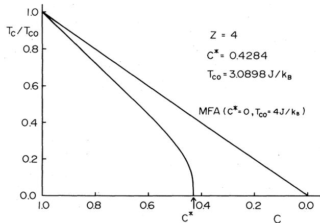
FIG. 6. Concentration dependence of the Curie temperature for the diluted square lattice. For comparison, the MFA result is also depicted.
