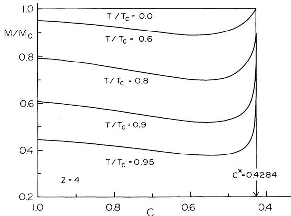
FIG. 8. Concentration dependence of the normalized magnetization for the diluted square lattice, in which the temperature is fixed at a given value.  $M_0$  is the magnetization at absolute zero.
