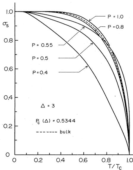
FIG. 10. Reduced magnetization curves of surface and bulk for  $\Delta=3$ . The critical value  $P_c(\Delta)=0.5344$  is determined from the relation  $\Delta_c(P)=3$ , as shown in Fig. 3.
