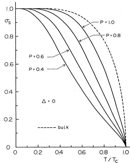
FIG. 9. Reduced magnetization curves of surface and bulk for  $\Delta=0$ , when the concentration  $P$  of magnetic atoms at the surface is change.
