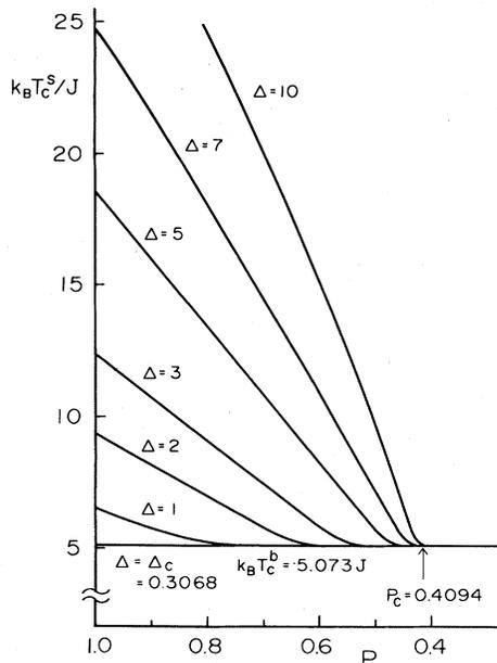
FIG. 4. Transition temperatures  $T_c^s$  for surface ordering are plotted as a function of surface concentration  $P$ . The values  $\Delta$  taken are larger than the critical value  $\Delta_c$ .
