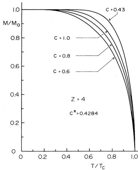
FIG. 7. Reduced magnetization curves vs the concentration  $C$  of magnetic atoms for the square lattice.
