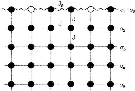
FIG. 1. Part of a two-dimensional cross section through a semi-infinite Ising lattice. Black points denote lattice positions, which are occupied by spins  $\mu_i = \pm 1$ . White points are nonmagnetic atoms. Full lines indicate exchange coupling  $J$ , while wavy lines indicate surface exchange couplings  $J_s = (1 + \Delta)$ .
