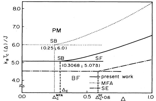
FIG. 2. Phase diagram in the  $(T, \Delta)$  space for the simple cubic Ising model with  $P=1$  and enhanced surface coupling  $J_s = J(1 + \Delta)$ . For comparison, the MFA and SE results (Refs. 1 and 3) are also plotted as a function of  $\Delta$ . The paramagnetic, bulk-ferromagnetic, and surface-ferromagnetic phases are indicated by PM, BF, and SF, respectively.
