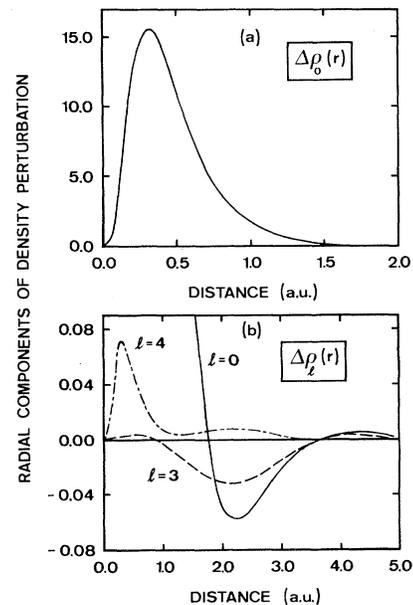
FIG. 3. (a) The  $l=0$  component of the self-consistent change  $\Delta\rho(\vec{r})$  in charge density for Si:Cu in an  $a_1$  Kubic-harmonics expansion. (b) An enlarged view of the three lowest nonzero radial  $l$  components of  $\Delta\rho(\vec{r})$ .
