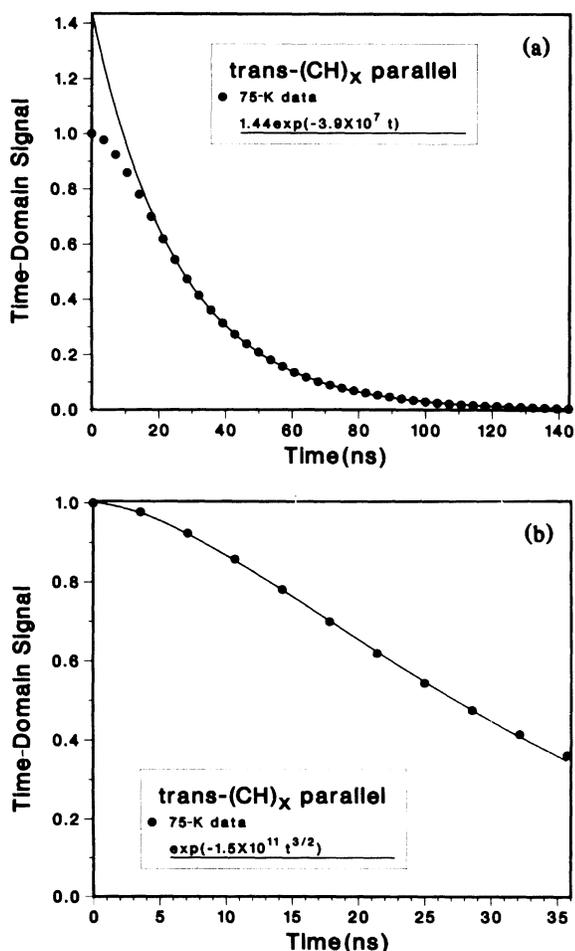
FIG. 1. (a) Time-domain signal at 75 K and its best fit for the tail portion. The data show an exponential decay tail for  $t > 20$  ns which indicates an off-chain hopping rate of about  $5 \times 10^7 \text{ s}^{-1}$ . (b) Short-time behavior of the time-domain signal at 75 K and its best fit. The characteristic  $t^{3/2}$  dependence in the exponent is due to the one-dimensional diffusion process.
