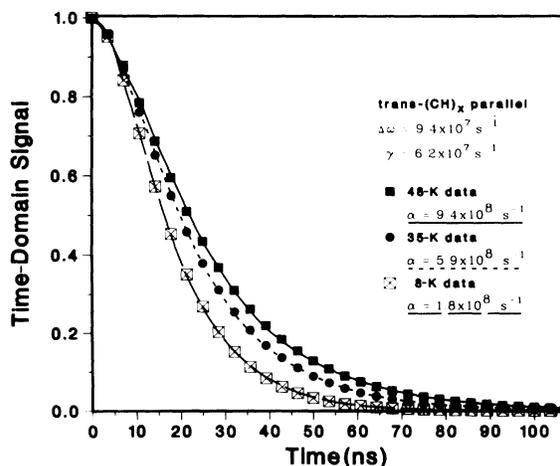
FIG. 2. Time-domain signals at three low temperatures and their best fits.  $\gamma$  is the off-chain hopping rate and  $\alpha$  is the on-chain diffusion rate. The observed hyperfine field  $\Delta\omega$  is smaller than that of localized spin and serves as evidence for spin delocalization.
