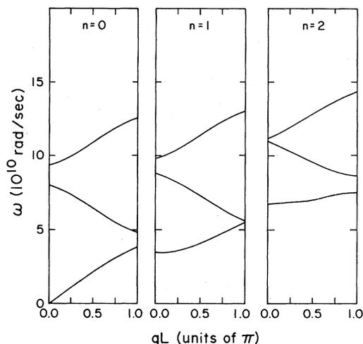
FIG. 7. Dispersion relations for the first three standing modes in the slab geometry of Fig. 2. Note the gaps at the zone edges. Calculations are performed with  $d_1=1000 \text{ \AA}$  of Nb and  $d_2=500 \text{ \AA}$  of Cu. The thickness of the slab is  $2000 \text{ \AA}$ .
