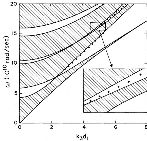
FIG. 10. Dispersion curves for the semi-infinite layered structure shown in Fig. 3 but with  $c_t > c'_t$ . Dotted lines show the surface modes. Shaded areas are the regions where bulk waves propagate. Calculations performed with  $d_1 = 1000 \text{ \AA}$  of Cu and  $d_2 = 500 \text{ \AA}$  of Nb.
