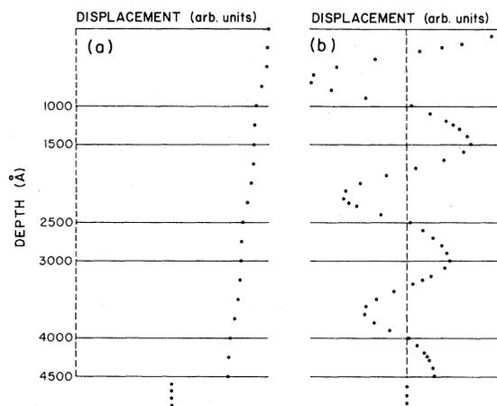
FIG. 9. Displacement patterns for surface modes. (a) shows the displacement of the surface wave at  $k_3 d_1=0.5, \omega=1.12 \times 10^{10} \text{ rad/sec}$  and (b) shows the displacement for the surface wave at  $k_3 d_1=0.5, \omega=8.76 \times 10^{10} \text{ rad/sec}$ .
