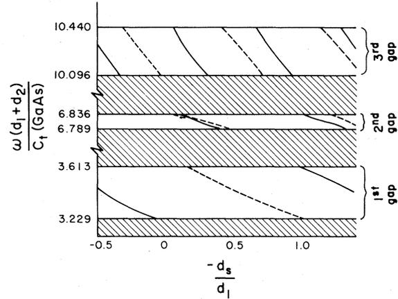
FIG. 11. Dispersion curves at  $k_3 = 0$  for the structure shown in Fig. 5. Shaded regions show the frequency range for propagation of bulk waves. Solid lines show the surface waves for a GaAs/AlAs structure when GaAs is on the surface. Dashed lines show the surface modes of a GaAs/AlAs structure when AlAs is the surface layer.
