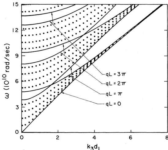
FIG. 6. Dispersion relation for transverse elastic waves propagating in the infinitely extended layered structure shown in Fig. 1. Calculations are performed with  $d_1 = 1000 \text{ \AA}$  of Nb and  $d_2 = 500 \text{ \AA}$  of Cu.
