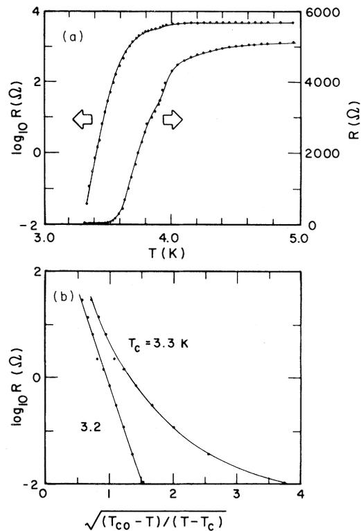
FIG. 1. (a) Resistive transition  $R$  ( $\Omega$ ) vs  $T$  (K) for sample no. 4, shown on a linear and a log scale. (b) Fit of the data from (a) for  $T < 3.5$  K to the theoretical expression Eq. (40), using  $T_{c0}=3.6$  K, and taking  $T_c=3.3$  K (right) and  $T_c=3.2$  K (left). The curve on the right is a guide to the eye; the straight line on the left corresponds to  $A=0.5$  and  $b=16.6$ .
