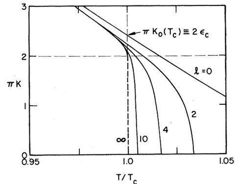
FIG. 6. Temperature dependence of the theoretical quantity  $\pi K(l, T) [=a(T) - 1]$  for several fixed values of the scale  $l$ . The same parameters are used as for Fig. 5. The line  $l=0$  corresponds to the bare, unrenormalized interaction  $\pi K_0$ ; the curve for  $l = \infty$  to the fully renormalized  $\pi K_R(T)$ .
