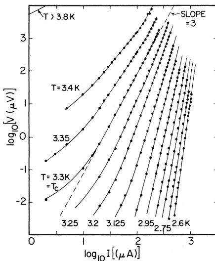
FIG. 2. Low-temperature  $I$ - $V$  curves for sample no. 4, on a log-log plot, for various fixed temperatures. The dashed line with slope = 3 corresponds to  $T_c$ .
