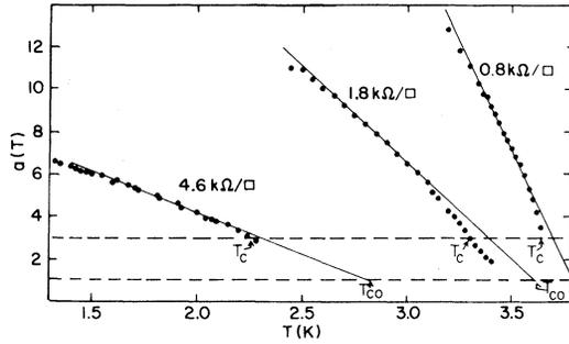
FIG. 3. Temperature dependence  $a(T)$  of the exponent from the low-temperature  $I$ - $V$  curves, for samples nos. 1, 4, and 5 (left to right). The straight lines  $a_{\text{lin}}(T)$  are drawn to fit the data below the critical region close to  $T_c$  [determined by  $a(T_c)=3$ ], and  $a_{\text{lin}}(T_{c0})=1$  determines  $T_{c0}$ .
