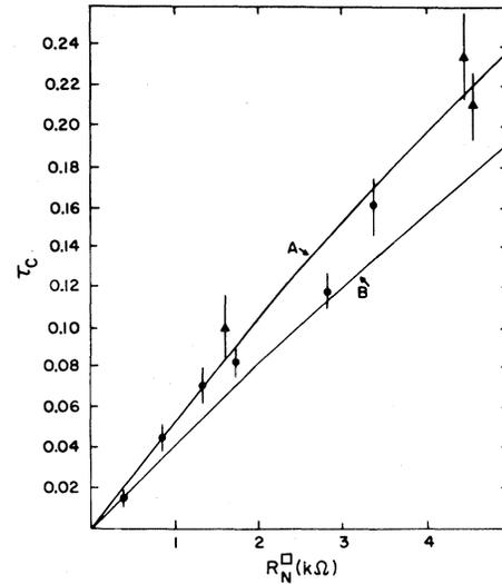
FIG. 4. Dependence of transition width  $\tau_c = 1 - T_c/T_{c0}$  on the normal-state sheet resistance  $R_N^{\square}$  for nine samples. The vertical error bars represent the uncertainty in determining  $T_{c0}$  by extrapolation. Curves A and B are theoretical curves using Eq. (37). Curve A uses a parameter  $\epsilon_c = 1.2$ , and curve B,  $\epsilon_c = 1.0$ , i.e., the result of BMO (Ref. 3).
