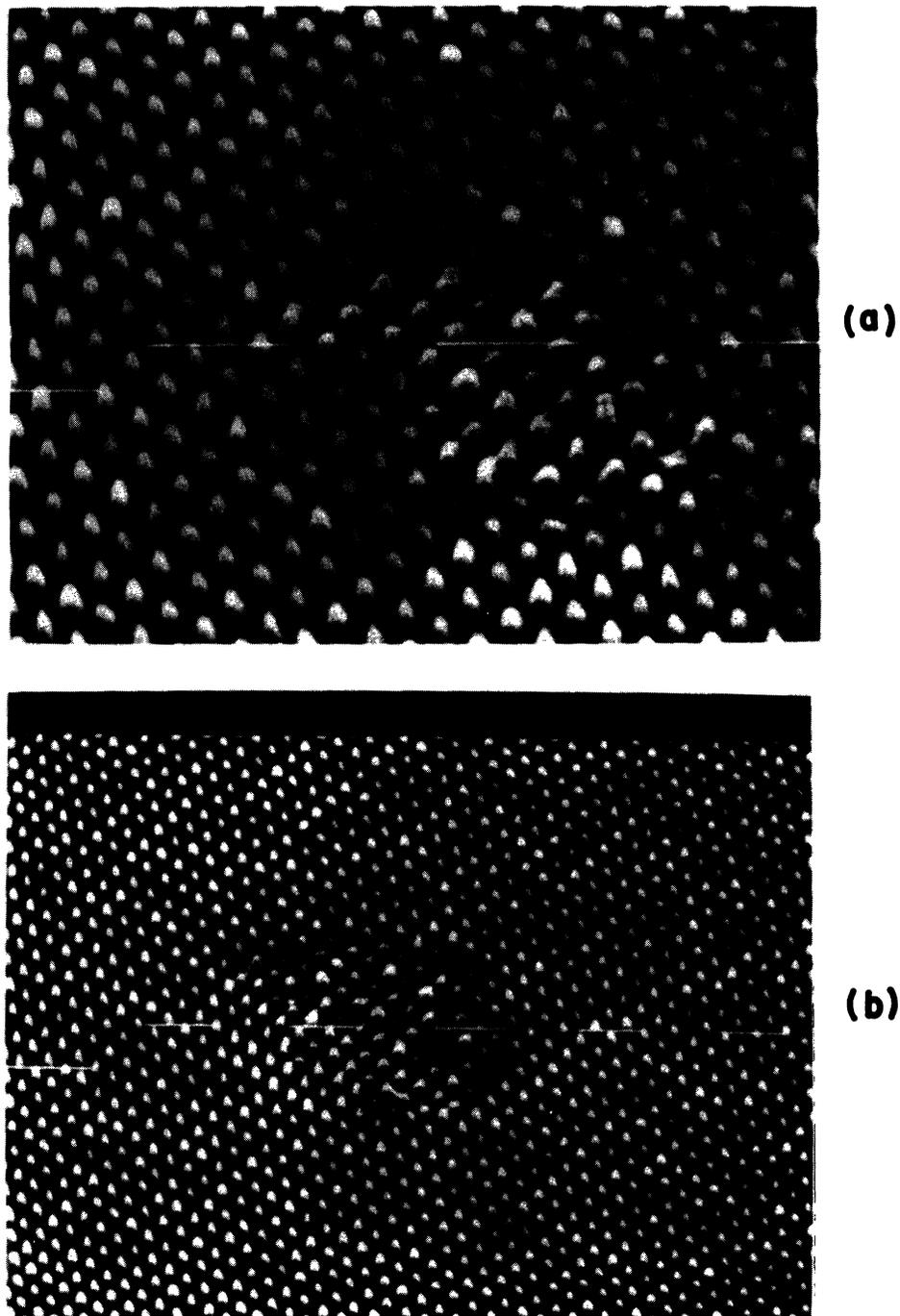
FIG. 4. Scanning electron micrographs of our sample after exposure to the two laser beams (5 mW average power each) focused on a  $8\text{-}\mu\text{m}$ -diameter spot. (a) After 1 min exposure, (b) after 2 min exposure, and (c) after 3 min exposure.
