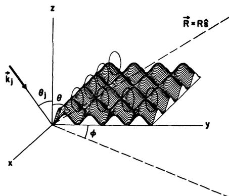
FIG. 1. Geometry of our samples and configuration of FWM. Silver particles are approximately shaped as ellipsoids of revolution with semiaxes  $b=1500$  Å and  $a=500$  Å. They are arranged on a planar double-square array of silicon-oxide microposts. Incident wave vectors are  $\vec{k}_j$  and the direction of observation given by the vector  $\vec{R}$  is  $R\hat{s}$ .
