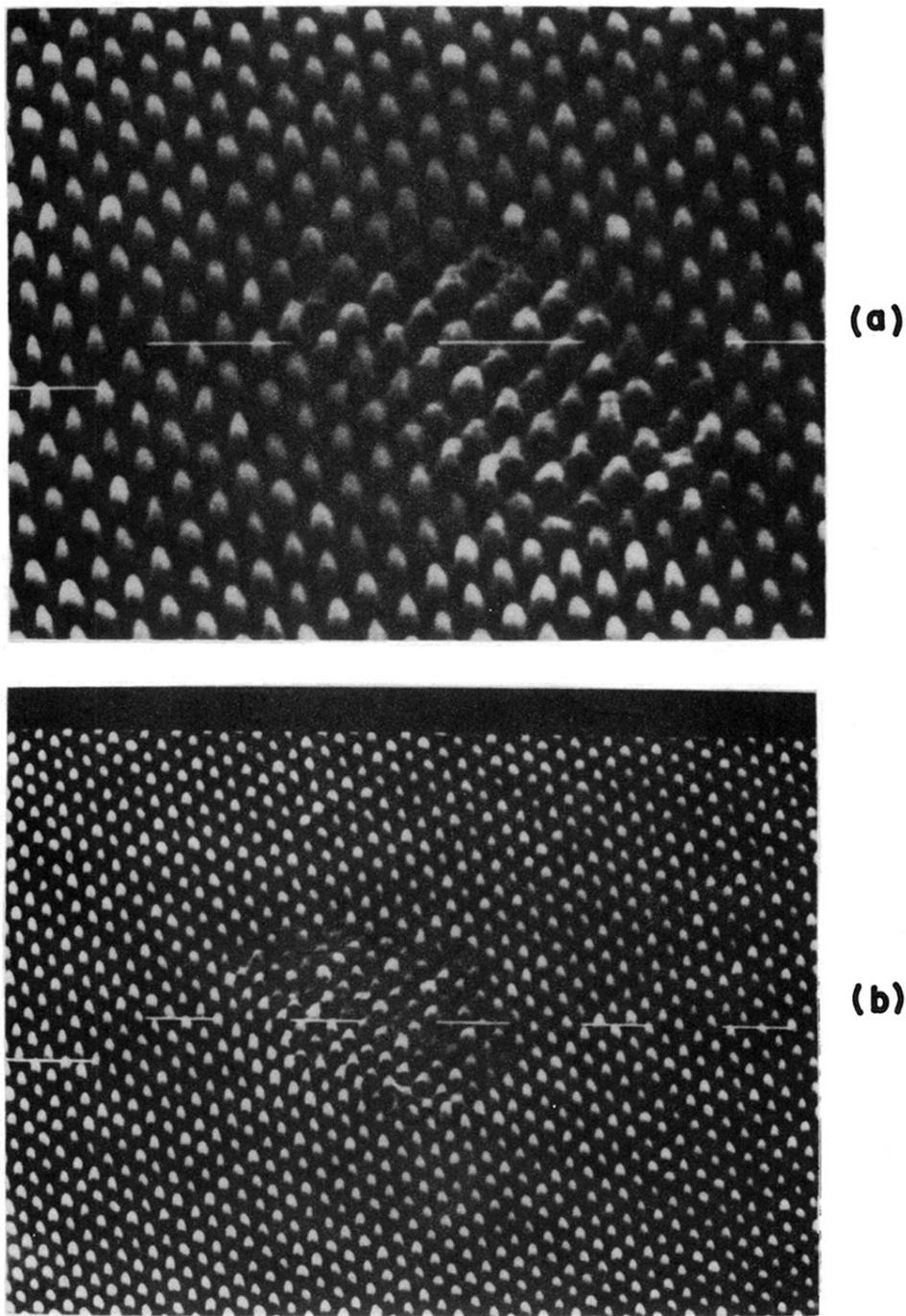
FIG. 4. Scanning electron micrographs of our sample after exposure to the two laser beams ( 5 mW average power each) focused on a 8- $\mu$ m-diameter spot. (a) After 1 min exposure, (b) after 2 min exposure, and (c) after 3 min exposure.
