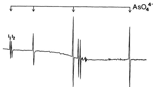
FIG. 1. ESR spectrum of the  $\text{AsO}_4^{4-}$  free radical in  $\text{KD}_2\text{PO}_4$ -5 mol %  $\text{KH}_2\text{AsO}_4$  (DKDP-KDA) at 82 K with the  $^{75}\text{As}$  hyperfine transitions indicated by arrows, showing the line intensities  $I_1$  and  $I_2$  of the split lowest-field hyperfine component. Additional lines arising from other paramagnetic species also appear in the center of the spectrum ( $\vec{H} \parallel c$ ,  $\vec{H} \parallel X$  or  $Y$ ).
