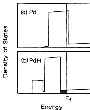
FIG. 9. Schematic DOS for (a) Pd and (b) PdH. (a) Pd: The DOS has contributions from the d states which in the Friedel model is a constant over a range equal to the width of the d bands. They can accommodate a total of ten electrons. The s bands have a free-electron-like DOS and contribute \gamma electrons up to the d -band edge. (b) PdH_x : The DOS in the strong bonding model has three main regions: (i) A low-lying bonding band with 2x electrons; (ii) the " d bands" which can hold 10 + \gamma - \alpha x electrons; (iii) a total of \delta(x) electron states that are occupied above the d -band edge (shaded region).
