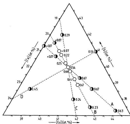
FIG. 2. Inductively determined  $T_c$  values (midpoint) of the samples. Half-filled circles indicate two or three phase samples detected on heavily overexposed Guinier films.
