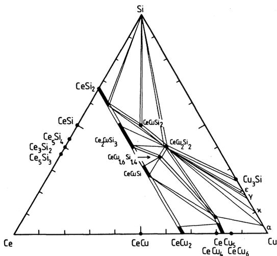
FIG. 1. Partial phase diagram of Ce-Cu-Si by Bodak *et al.* (Ref. 7).
