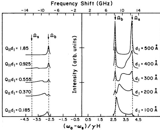
FIG. 9. Light-scattering spectrum from a LUCS structure of alternating layers of Ni and Mo. Here  $d_1 = d_2$ , and the applied field is  $H_0 = 1$  kG. For the geometry of the light scattering ( $\theta_0 = 74^\circ$ ,  $\theta_s = 84^\circ$ ), there is a large asymmetry between the intensity of the Stokes side and on the anti-Stokes side.
