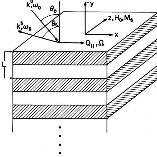
FIG. 6. Geometry of the light-scattering experiment. The incident light, with wave vector  $\vec{k}^{(0)}$  and frequency  $\omega_0$ , strikes the surface at an angle  $\theta_0$  with respect to the surface normal. The scattered light has wave vector  $\vec{k}^{(s)}$  and frequency  $\omega_s$ .
