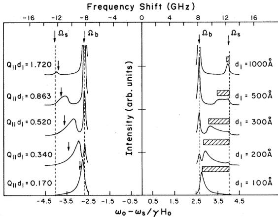
FIG. 7. Light-scattering spectrum from a LUCS structure of alternating layers of Ni and Mo for different values of  $d_1$ . Here  $d_1 = d_2$ . The box over each spectrum on the Stokes side gives the frequency range of bulk spin waves in the layered structure. The arrow over each spectrum on the anti-Stokes side gives the frequency of a surface spin wave on an isolated film of thickness  $d_1$ .
