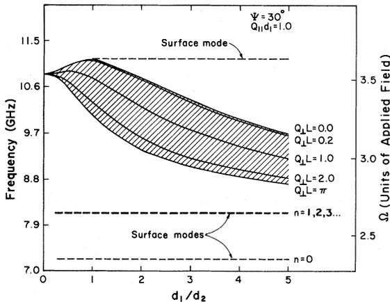
FIG. 4. Frequency of various modes vs the ratio  $d_1/d_2$ . Bulk modes of the stack are shown with a solid line, surface modes of the stack have a dashed line. Modes with  $n \geq 1$  lie very close in frequency, and cannot be resolved on the scale of the graph.
