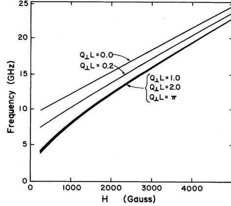
FIG. 5. Frequency of different bulk modes vs applied field.
