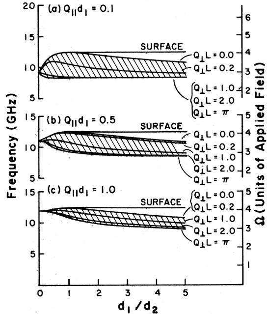
FIG. 3. Frequency of various modes vs the ratio  $d_1/d_2$ . Bulk modes of the stack are shown with a shaded region the surface modes are shown by a solid line.
