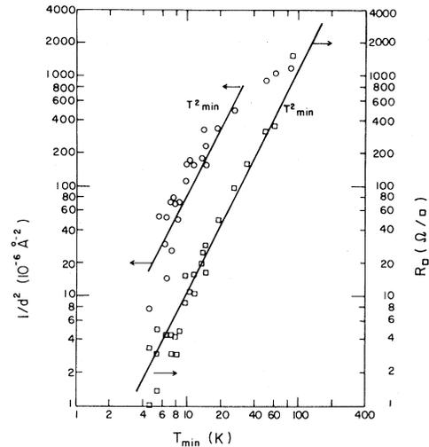
FIG. 5. Behavior of  $T_{\text{min}}$ , the temperature at which the resistance minimum occurs, for different film resistances  $R_0$ . The relation between  $T_{\text{min}}$  and  $d^{-2}$  is also shown where  $d$  is the film thickness.  $T_{\text{min}}$  saturates at 5 K owing to magnetic impurities which have a Kondo temperature at this temperature.
