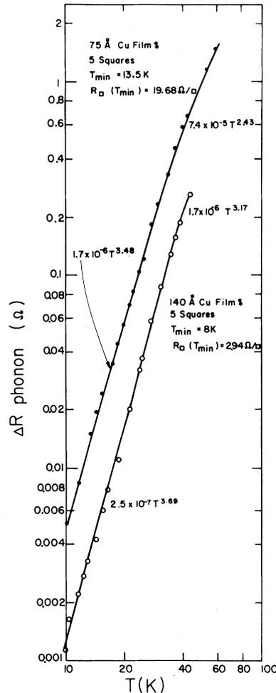
FIG. 3. Temperature dependence of  $\Delta R_{\text{phonon}} = aT^q$  for two different Cu films. The exponent  $q$  takes on a typical value of 3.6 in the 10- to 20-K temperature interval. At higher temperatures  $q$  decreases to about 2.5.
