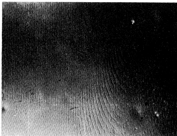
FIG. 13. Photograph of a portion of the Ge surface after being hit by 10 pulses of 1.06- \mu\text{m} , p -polarized radiation. Note how the fanlike pattern emanating from the localized defect continuously transforms into the parallel, type- c fringes which eventually dominate.
