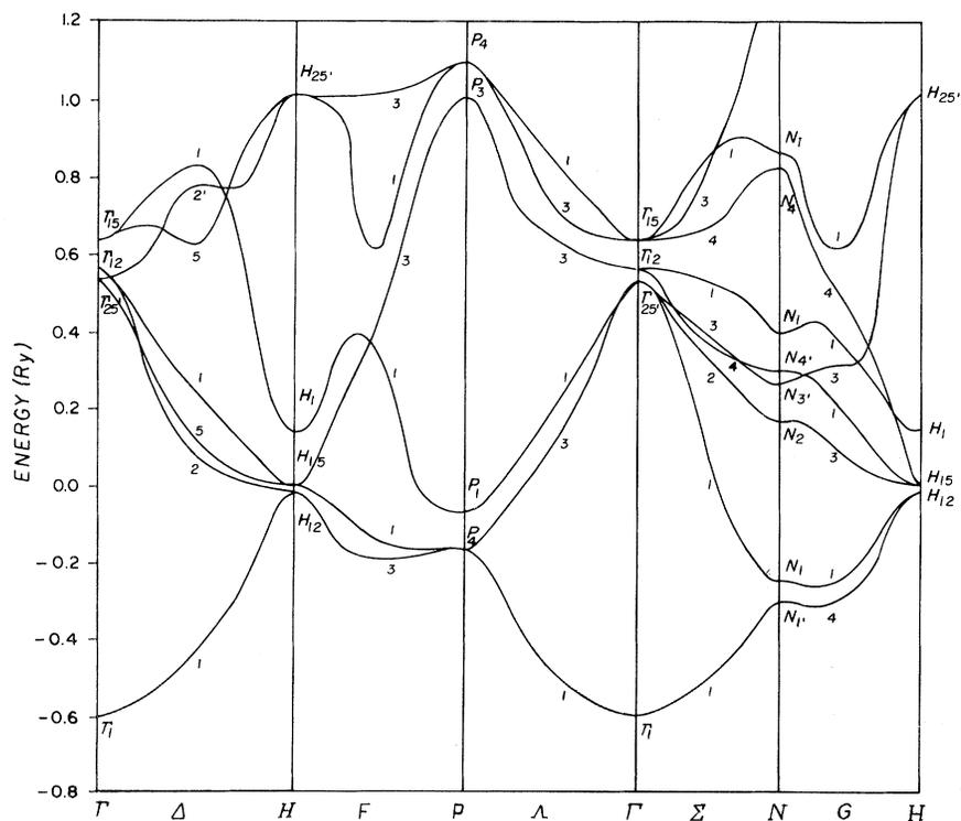
FIG. 3. Energy-band structure of bcc sodium obtained from the VCM calculations.
