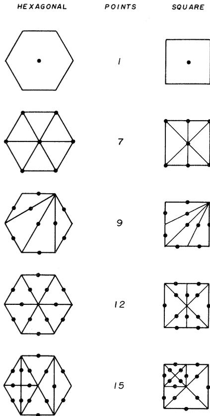
FIG. 2. Different sets of points used to perform the cellular calculations. The square and the hexagon represent the two kind of polyhedral faces.
