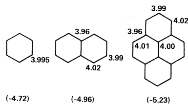
FIG. 8. Clusters modeling the graphite lattice with the calculated valence charge indicated. Binding energies are reported for each structure in units in eV/atom enclosed in parenthesis.
