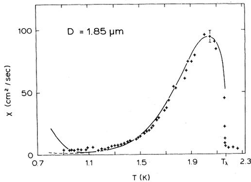
FIG. 4. Thermal diffusivity  $\chi$  in dependence on temperature for a channel width of  $D=1.85 \mu\text{m}$ . The solid line represents the result of the thermohydrodynamic theory according to Eq. (6), and the dashed line is calculated on the basis of a kinetic theory (Ref. 33) by taking mean-free-path effects of the elementary excitations into account.
