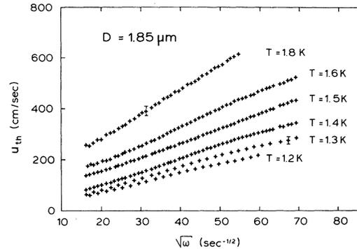
FIG. 3. Phase velocity of the thermal wave  $u_{\text{th}}$  as a function of the square root of the angular frequency  $\omega$  for a plate separation of  $D=1.85 \mu\text{m}$  and at various temperatures between 1.2 and 1.8 K.
