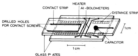
FIG. 2. Schematic diagram of the apparatus used to detect the thermal wave.
