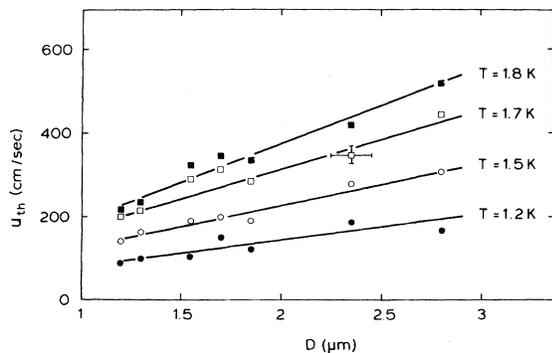
FIG. 6. Phase velocity of the thermal wave  $u_{\text{th}}$  plotted against the width of the plane-parallel slit  $D$  at the temperatures  $T=1.2, 1.5, 1.7,$  and  $1.8 \text{ K}$ . The straight lines are fitted to the data and reveal in consistency with the theory according to Eq. (2) a linear relationship between the phase velocity and the slit width.
