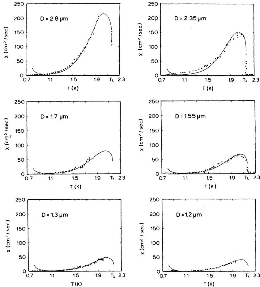
FIG. 5. Thermal diffusivity as a function of temperature at the channel widths  $D=2.8, 2.35, 1.7, 1.55, 1.3,$  and  $1.2 \mu\text{m}$ . The solid lines indicate the results of the theory according to Eq. (6), and the dashed lines are calculated by means of a kinetic theory (Ref. 33).
