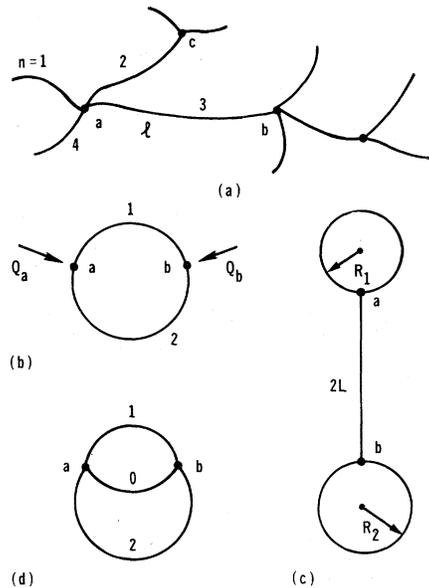
FIG. 1. Shown are (a) general network, with nodes  $a, b$ , and  $c$ ; (b) a loop with two nodes and current injection through a velocity field  $Q_a = -Q_b$ ; (c) the bola, consisting of two "lassos"; (d) the Wheatstone bridge.
