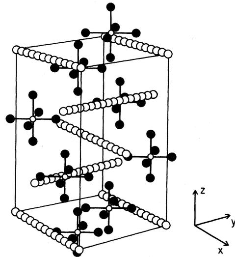
FIG. 4. Structure of  $Hg_{3-\delta}AsF_6$ . The Hg atoms on the chains are shown schematically. Above 120 K the Hg atoms form a fluid with no long-range order.
