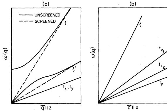
FIG. 3. Phonon dispersion for a uniaxial incommensurate polar material. (a)  $q$  along unique axis. (b)  $q$  perpendicular to unique axis. Subscripts indicate displacement direction.
