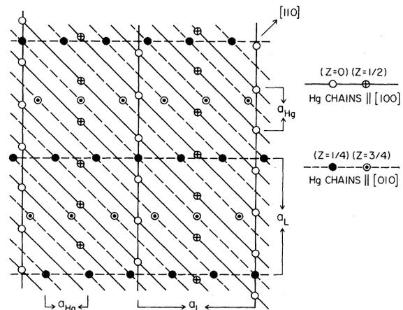
FIG. 5. Ordered structure of  $Hg_{3-\delta}AsF_6$  below 120 K.
