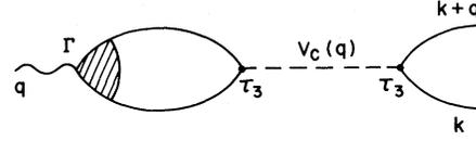
FIG. 4. Screening of the vertex via the Coulomb potential  $V_c$  in a charged superconductor.
