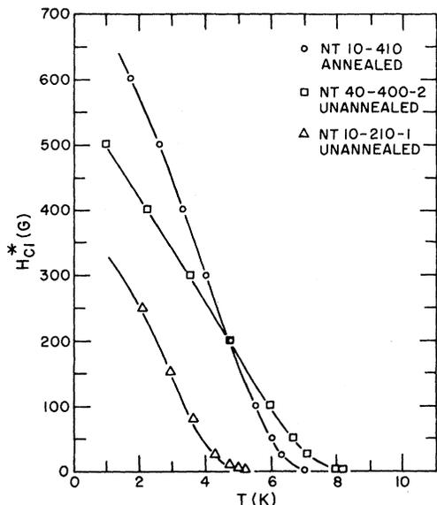
FIG. 7. Field  $H_{c1}^*$  vs temperature for several samples of Th-Nb. Sample NT 10-210-1 has  $t = 76 \text{ \AA}$  and sample NT 40-400-2 has  $t = 145 \text{ \AA}$ .
