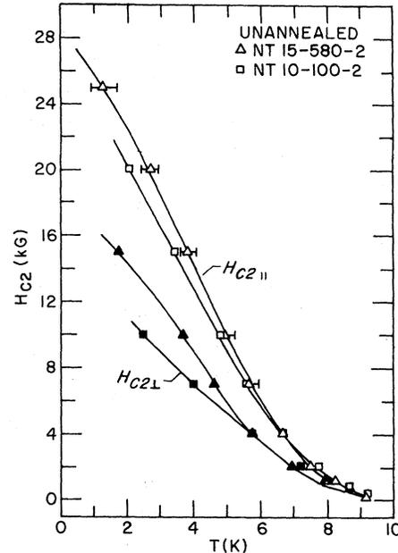
FIG. 3. Upper critical field vs temperature for two unannealed samples for both the case of the field parallel and the case of the field perpendicular to the filaments. Error bars show the points of 20% and 80% of the normal-state resistance for sample NT 15-580-2. Sample NT 15-580-2 has  $t=210$  Å and sample NT 10-100-2 has  $t=36$  Å.
