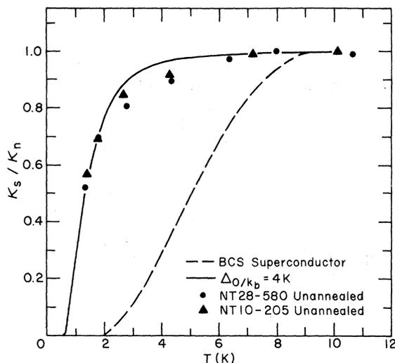
FIG. 8. Ratio of the thermal conductivity in the superconducting state to that in the normal state for two unannealed Th-Nb samples. Dashed line is the Bardeen-Rickaysen-Tewordt calculation for an ordinary BCS superconductor ( $2\Delta_0/kT_c = 3.53$ ). Solid line is a similar calculation for a smaller energy gap. Sample NT 28-580 has  $t = 210$  Å and sample NT 10-205 has  $t = 74$  Å.
