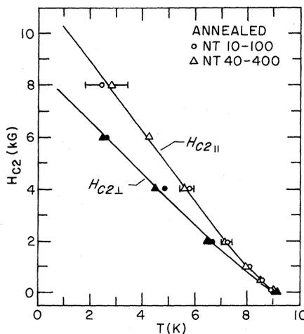
FIG. 4. Upper critical field vs temperature for two annealed samples for both the case of the field parallel and the case of the field perpendicular to the long dimension of the wire. Error bars show the points of 20% and 80% of the normal-state resistance for sample NT 10-100.
