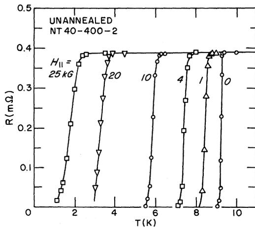
FIG. 1. Resistance vs temperature in several magnetic fields for an unannealed Th-Nb sample with  $t = 145$  Å. Direction of the current and magnetic field are parallel to the filaments.
