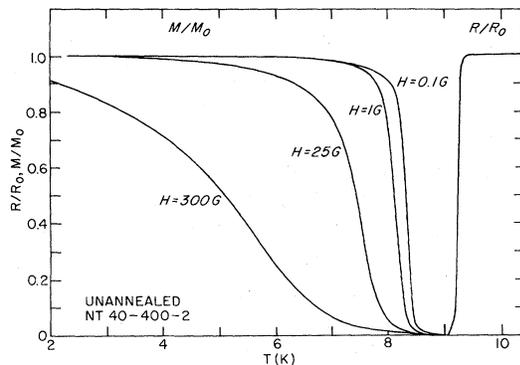
FIG. 5. Normalized resistance and dc magnetization vs temperature for an unannealed sample of Th-Nb having  $t=145$  Å. Magnetization measurements were made for several values of the field applied parallel to the filaments.
