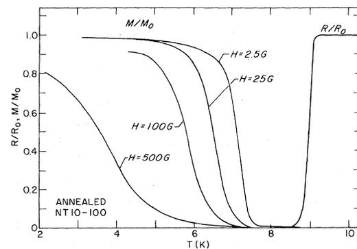
FIG. 6. Normalized resistance and dc magnetization vs temperature for an annealed Th-Nb sample.
