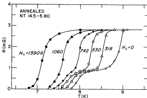
FIG. 2. Resistance vs temperature in several magnetic fields for an annealed sample of Th-Nb. Only a few of the annealed samples showed a plateau in zero field.
