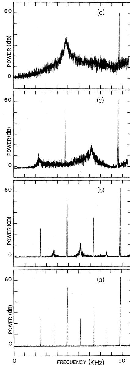
FIG. 3. Observed power spectral density  $S(f)$  under same conditions as Fig. 2, with driving frequency  $f = 96$  kHz: (a) no added noise, sharp subharmonics  $f/2$  to  $f/16$  displayed; (b) added noise  $\sigma_m = 1.4 \times 10^{-4}$ , removes sharp  $f/16$  components; (c)  $\sigma_m = 8.7 \times 10^{-4}$ , removes sharp  $f/8$  components; (d)  $\sigma_m = 5.5 \times 10^{-3}$ , removes sharp  $f/4$  component.
