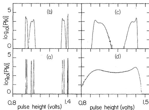
FIG. 2. Observed  $\log_{10}P(V_c)$  vs  $V_c$  for varactor voltage  $V_c$  of nonlinear oscillator, bifurcated to subharmonic  $f/16$ : (a) added noise voltage  $\sigma_m = 0$ ; (b)  $\sigma_m = 1.4 \times 10^{-4}$ ; (c)  $\sigma_m = 8.7 \times 10^{-4}$ ; (d)  $\sigma_m = 5.5 \times 10^{-3}$ .
