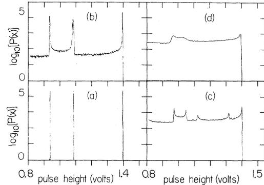
FIG. 5. Observed  $\log_{10}P(V_c)$  vs  $V_c$ : (a) at onset of period-5 window with no added noise; (b) added noise  $\sigma_m = 1.1 \times 10^{-4}$ ; (c) chaotic region ( $\lambda \approx 3.7$ ) with no added noise  $\sigma_m = 1 \times 10^{-3}$ .
