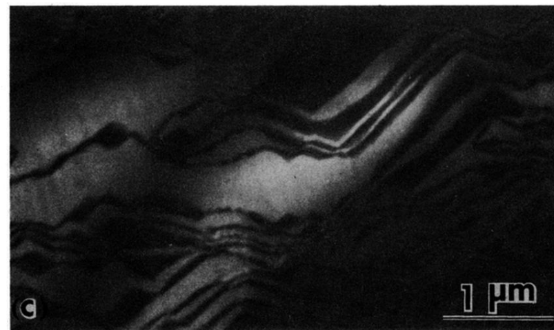
FIG. 15. (a)–(c) Triple- q imaging at 86 K in the “hexagonal” phase on cooling. Image characteristics are similar to the orthorhombic domains in the commensurate phase (Fig. 1); i.e., a domain appears dark for only one particular imaging direction and appears bright for the other two imaging directions.
