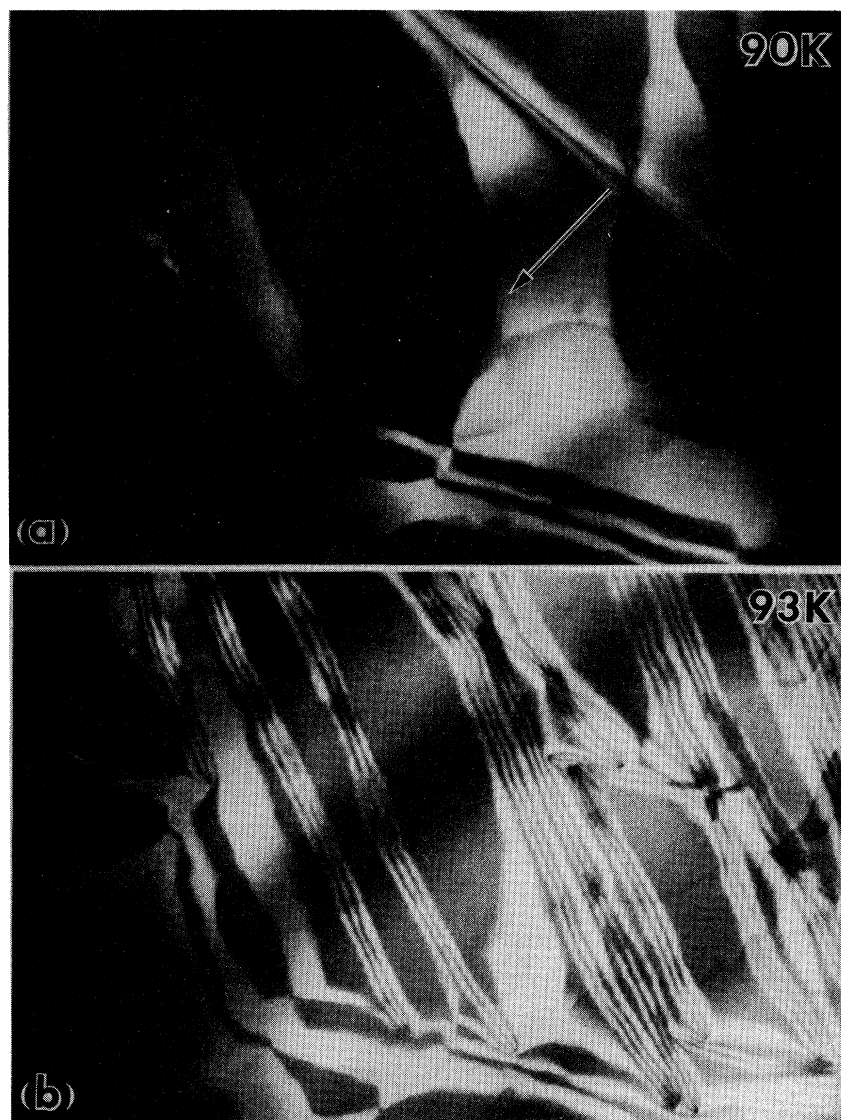
FIG. 3. Evolution of the stripe phase from the orthorhombic commensurate phase. Imaging direction is also indicated by the arrow.
