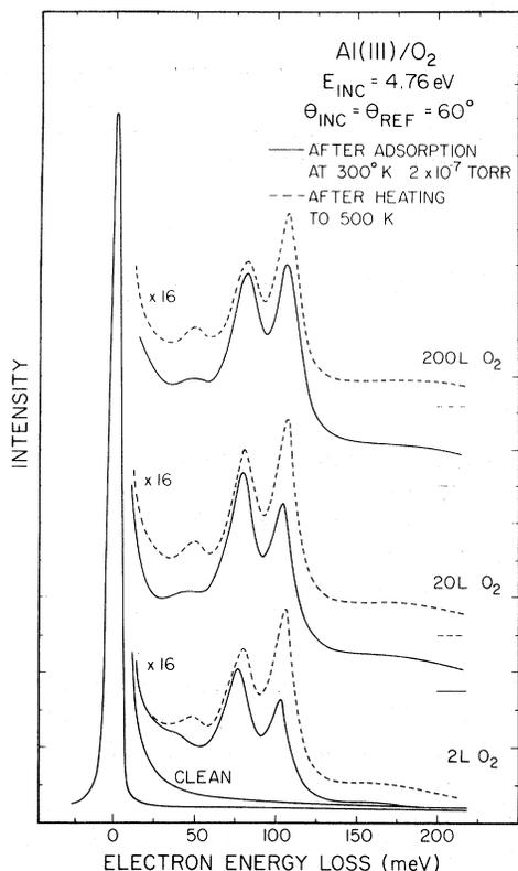
FIG. 1. EELS spectra for Al(111) exposed at 300 K to 2, 20, and 200 L of oxygen at  $2 \times 10^{-7}$  Torr (solid curves) corresponding spectra after heating to 500 K (dashed curves). Scattering angles,  $\theta$ , are measured from the surface normal. Electron impact energy  $E_{\text{inc}} = 4.76$  eV. Baselines for each curve are indicated to the right. All spectra were normalized so that elastic peak intensities were equal and scale factors indicated are relative to the elastic peak.
