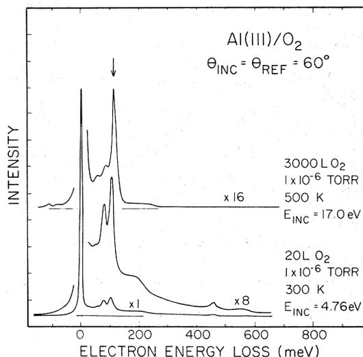
FIG. 3. Lower EELS spectrum corresponds to surface and subsurface oxygen after 12 h. Upper EELS spectrum corresponds to Al<sub>2</sub>O<sub>3</sub>. Arrow shows position of dominant infrared absorption for Al<sub>2</sub>O<sub>3</sub> at 118 meV (940 cm<sup>-1</sup>) (Refs. 17 and 18). The peak at 463 meV corresponds to the O–H stretch of adsorbed OH groups.
