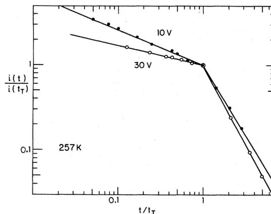
FIG. 3. Current transients in  $\log i$  vs  $\log t$  units normalized to their respective transit times for two applied voltages at a constant temperature.
