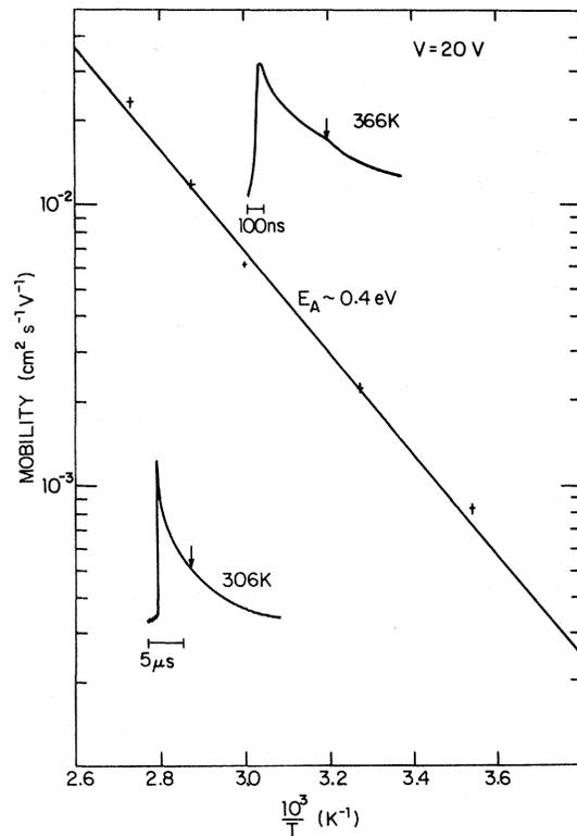
FIG. 12. Temperature dependence of the hole drift mobility. The sample thickness is  $4.6 \mu\text{m}$ . Representative photocurrent decays are shown in linear units.
