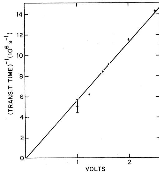
FIG. 5. Voltage dependence of the reciprocal transit time for a sample displaying nondispersive behavior.
