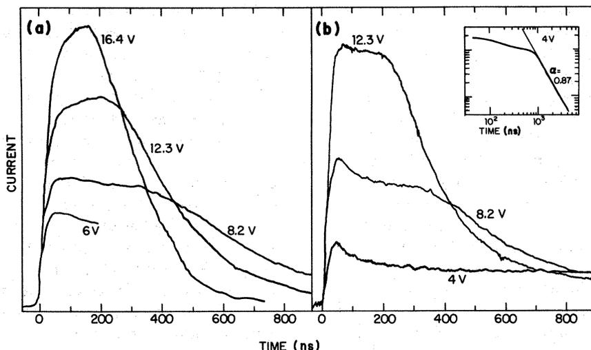
FIG. 6. Voltage dependence of the shape of the electron photocurrent transients at 300 K. (a) corresponds to a sample with a platinum top contact and (b) with Nichrome. The samples, prepared in the same sputtering run, are of somewhat different thicknesses.
