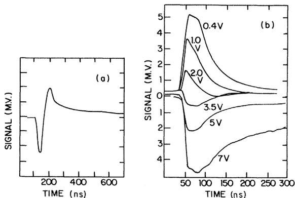
FIG. 11. Low forward-bias phototransients.
