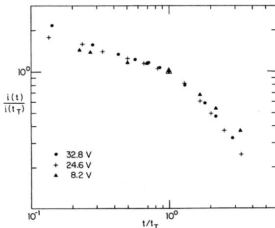
FIG. 8. Transient currents in units of  $\log i$  vs  $\log t$  at constant temperature for different applied voltages. The traces are normalized with respect to the transit time on the  $\log t$  axis.
