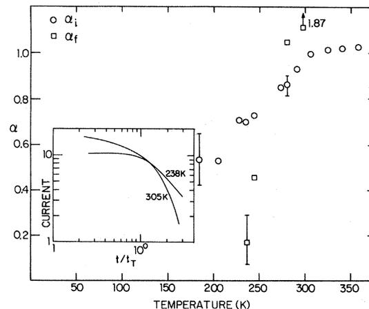
FIG. 9. Temperature dependence of the dispersion parameter  $\alpha$  obtained from the initial and final slopes of a  $\log i$  vs  $\log t$  representation of the photocurrent transients. The inset shows current traces in logarithmic units at two temperatures.
