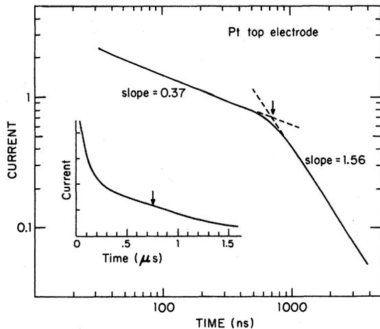
FIG. 1. Dispersive current transient in units of  $\log i$  vs  $\log t$  (main figure) and units of  $i$  vs  $t$  (inset). The arrow in the inset marks the position of the transient time obtained from the intercept of the tangents illustrated in the main figure. A field  $2.8 \times 10^4$  V/cm is present and the temperature of measurement is 257 K.
