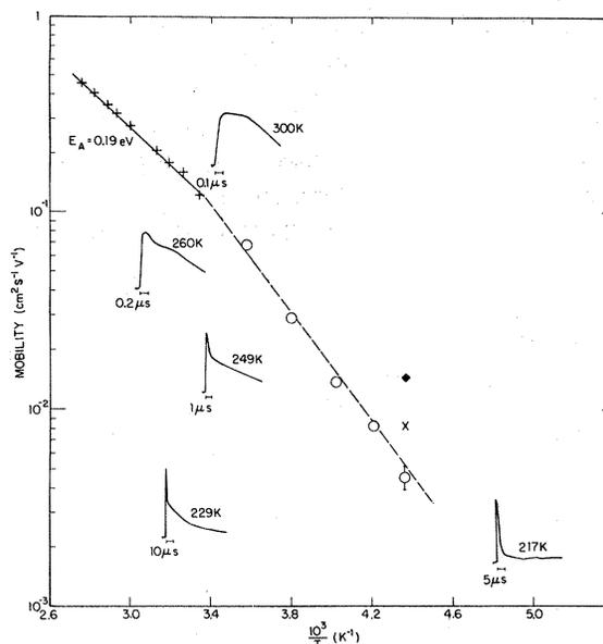
FIG. 7. Temperature dependence of the electron drift mobility for an applied electric field of  $1 \times 10^4$  V/cm (+ and O). Representative current transients observed at various temperatures are displayed in linear units. The field dependence of the mobility is shown at  $T = 230$  K (X and  $\blacklozenge$  refer to electric fields of  $3 \times 10^4$  and  $4 \times 10^4$  V/cm, respectively). The sample thickness is  $8.2 \mu\text{m}$ .
