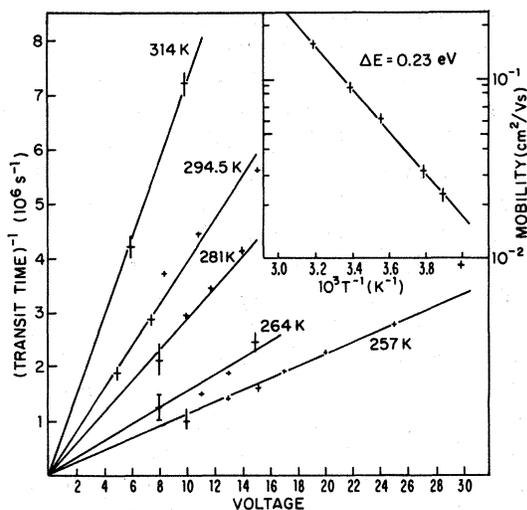
FIG. 2. Voltage dependence of the reciprocal transit time at several temperatures for the sample of Fig. 1. The inset shows the temperature dependence of the mobility calculated in the linear low-voltage region.
