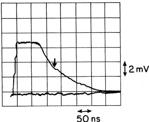
FIG. 4. Single-shot phototransients for a sample displaying nondispersive behavior. The sample thickness is 1.35  $\mu\text{m}$  and 1.5 V is applied across the sample.
