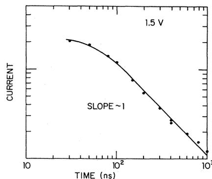
FIG. 10. Electron phototransients observed in samples which have greater than  $1 \times 10^{17} \text{cm}^{-3} \text{eV}^{-1}$  states at the Fermi level.
