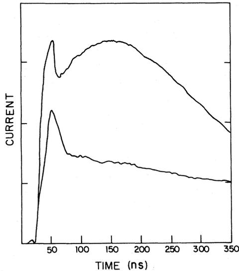
FIG. 13. Transient currents observed under high injection conditions in a nondispersive regime (upper trace) and dispersive regime (lower trace). The applied voltage and light intensities are the same for both traces.
