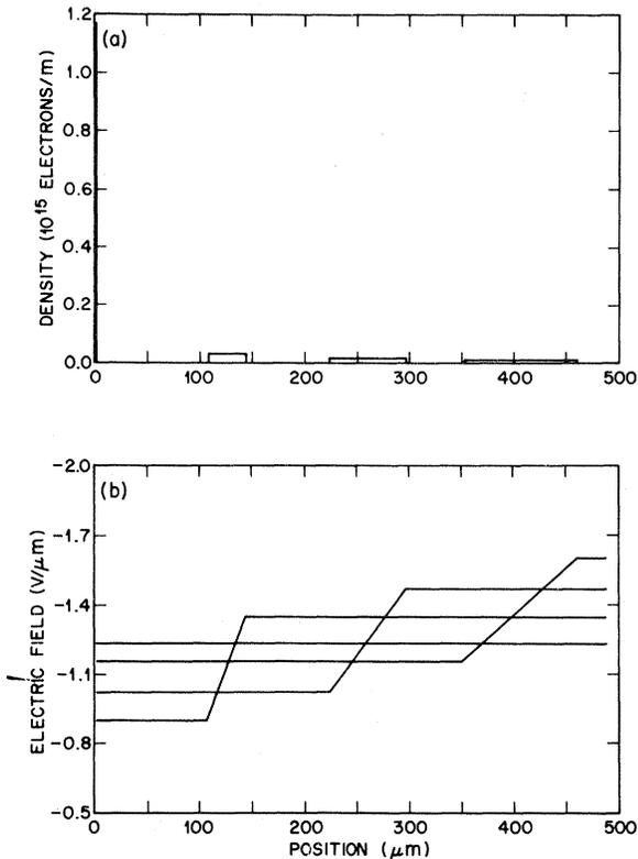
FIG. 5. (a) Density vs position at four different times. Conditions same as Fig. 4. (b) Electric field vs position for the same four times as in part (a).
