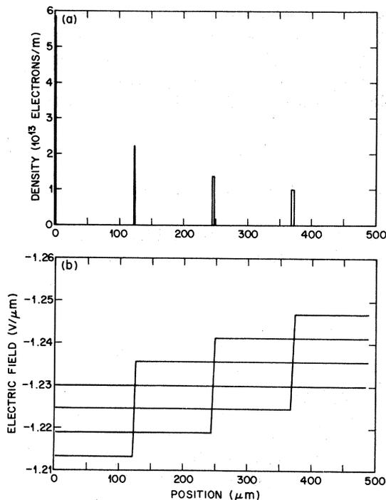
FIG. 2. (a) Density vs position at four different times. The conditions correspond to a particle measurement (Ref. 20), where  $a = 8.15 \times 10^{-6}$  m/s,  $L = 488$   $\mu\text{m}$ ,  $N = 5.85 \times 10^7$ ,  $v_0 = 3.65 \times 10^4$  m/s, and  $w_0 = 1.0$   $\mu\text{m}$ . (b) Electric field vs position for the same four times as in part (a).
