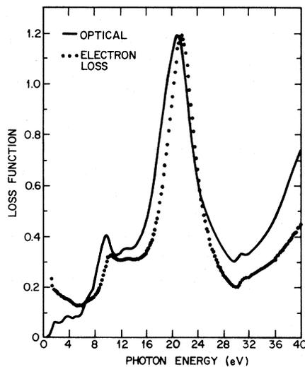
FIG. 1. Electron-energy-loss spectrum of pure Nb for  $q=0$ , and optical data from Ref. 5.
