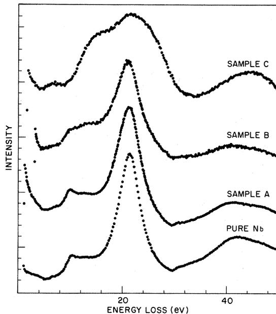
FIG. 5. Energy-loss spectra of Nb-O samples. Samples *A*, *B*, and *C* have superconducting transition temperature at 7.8, 5.5, and  $< 1.2$  K, respectively. For comparison, a loss spectrum of pure Nb (Fig. 1) is also included.
