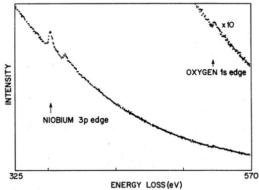
FIG. 4. Core-level spectra showing the existence of oxygen 1s excitation. Also shown are Nb 4p core excitations.
