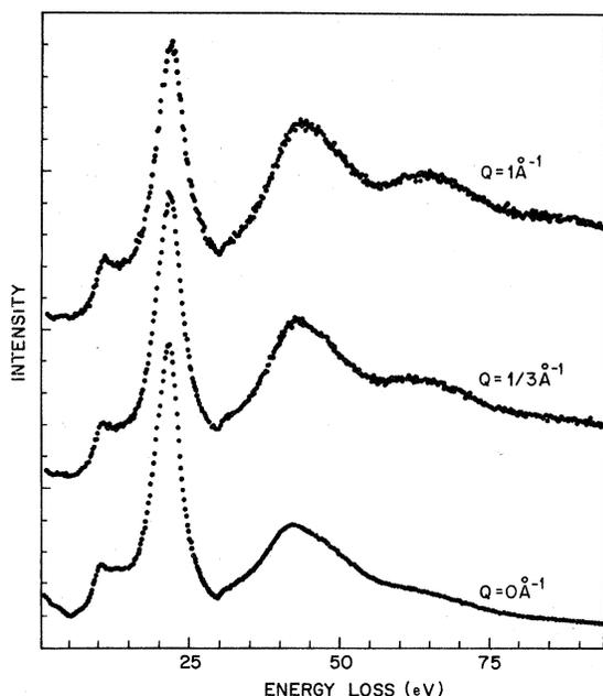
FIG. 2.  $q$  dependence of the energy-loss spectra of pure Nb.
