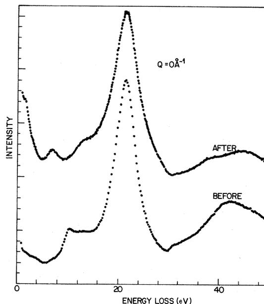
FIG. 3. Electron-energy-loss spectrum of a Nb foil before and after prolonged air oxidation.
