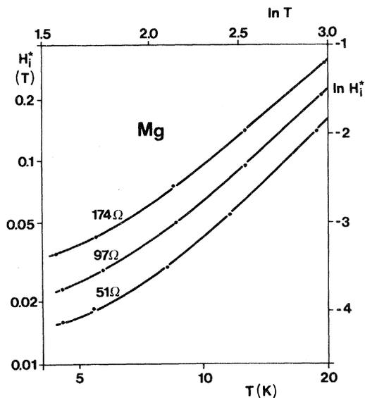
FIG. 2. Adjusted characteristic field  $H_i^*(T)$  as a function of temperature in a log-log plot for three Mg films.
