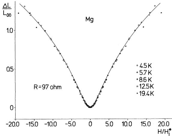
FIG. 1. Normalized conductance  $\Delta L/L_{00}$  of the Mg film as a function of the (normalized) magnetic field  $H/H_i^*(T)$  for different temperatures compared with the theory (full curve),  $L_{00} = \hbar/(2\pi^2 e^2)$ .
