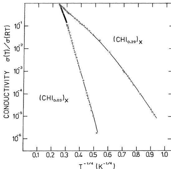
FIG. 1. Logarithm of the electrical conductivity normalized to room-temperature conductivity versus  $T^{-1/4}$  for  $(\text{CHI}_{0.03})_x$  and  $(\text{CHI}_{0.29})_x$ .
