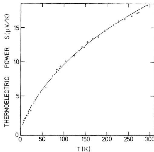
FIG. 2. Thermoelectric power of  $(\text{CHI}_{0.22})_x$  vs  $T$  from the data of Park *et al.*
