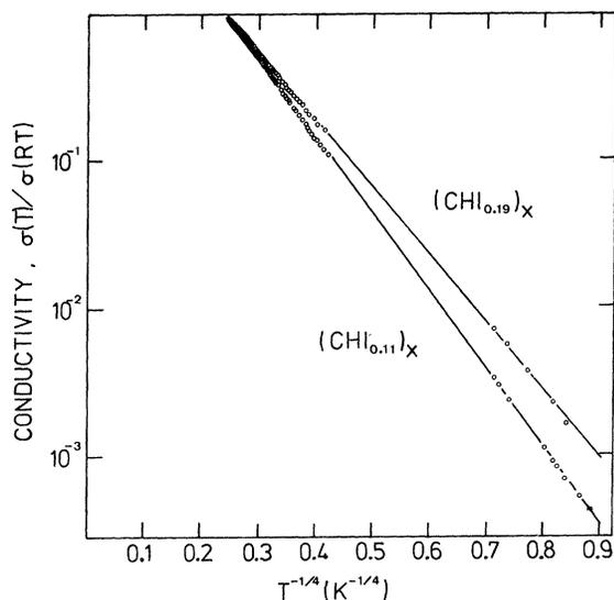
FIG. 3. Logarithm of the electrical conductivity normalized to room-temperature conductivity versus  $T^{-1/4}$  for  $(\text{CHI}_{0.11})_x$  and  $(\text{CHI}_{0.19})_x$ .
