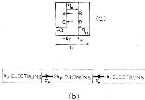
FIG. 1. (a) Normal and umklapp electron-phonon scatterings. The definitions of  $q_N$ ,  $q_U$ ,  $Q$ , and  $G$  are given in the text. (b) Momentum transfer for  $2k_F$  phonons in the commensurate phase from  $k_F$  and  $-k_F$  electrons via relaxation times  $\tau_N$  and  $\tau_U$ .
