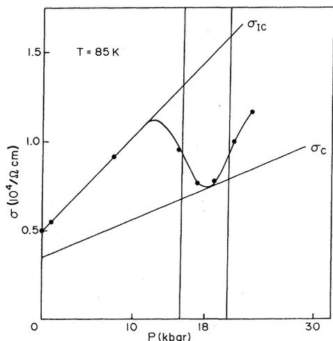
FIG. 2. Pressure dependence of  $\sigma_{\text{IC}}$  and  $\sigma_{\text{C}}$  at 85 K. The vertical lines define the range of "pressure commensurability" due to thermal smearing.
