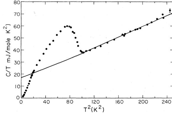
FIG. 3. Specific heat of  $\text{Nb}_3\text{Al}$  irradiated to a fluence of  $1.3 \times 10^{19} \text{ n/cm}^2$ .
