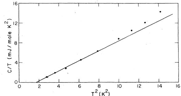
FIG. 5. Low-temperature specific heat of Nb<sub>3</sub>Al irradiated to a fluence of  $1.3 \times 10^{18}$  n/cm<sup>2</sup>.
