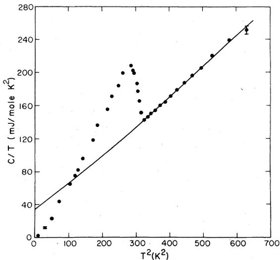
FIG. 2. Specific heat of  $\text{Nb}_3\text{Al}$  irradiated to a fluence of  $1.3 \times 10^{18} \text{ n/cm}^2$ .
