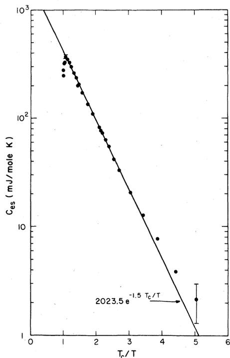
FIG. 8. Electronic specific heat in the superconducting state of  $\text{Nb}_3\text{Al}$  irradiated to fluence  $1.3 \times 10^{19} \text{ n/cm}^2$ .
