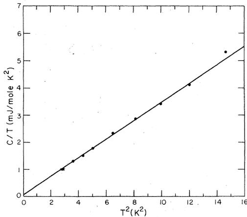
FIG. 4. Low-temperature specific heat of unirradiated Nb<sub>3</sub>Al.
