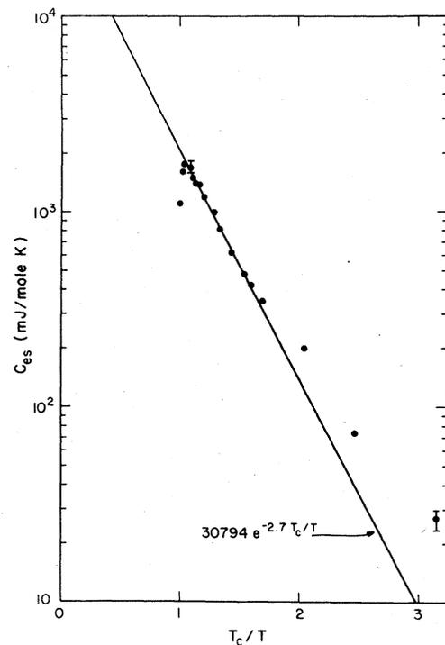
FIG. 7. Electronic specific heat in the superconducting state of Nb<sub>3</sub>Al irradiated to fluence  $1.3 \times 10^{18} n/cm^2$ .
