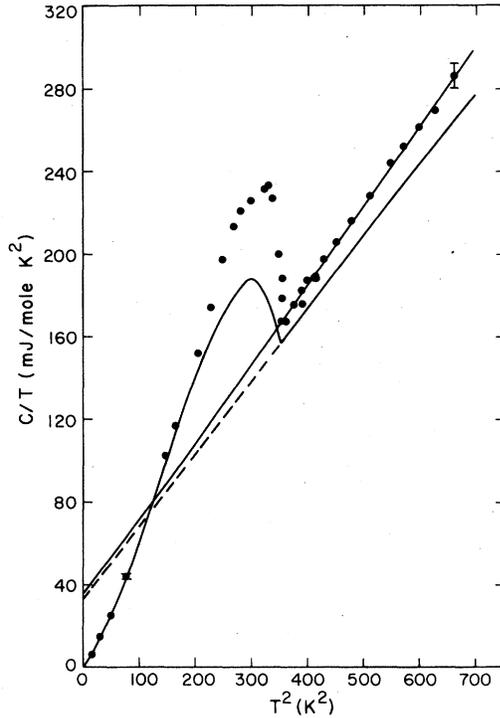
FIG. 1. Specific heat of unirradiated  $\text{Nb}_3\text{Al}$ . The lower curve is taken from Ref. 10 for comparison. The error bars on this figure and those following indicate the internal precision of  $\pm 2\%$  of the data.
