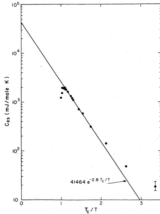
FIG. 6. Electronic specific heat of unirradiated Nb<sub>3</sub>Al in the superconducting state.
