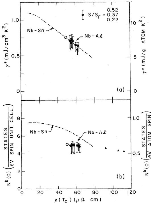
FIG. 3. (a) Electronic specific-heat coefficient  $\gamma^*$  vs  $\rho(T_c)$  and (b) band density of states at the Fermi level  $N^b(0)$  vs  $\rho(T_c)$ , for (○) bulk  $\text{Nb}_3\text{Al}$ , (●)  $\text{Nb-Al}$  this work, (---)  $\text{Nb-Sn}$  Ref. 16, and (▲)  $\text{Nb}_3\text{Al}$  radiation damaged with corrections described in the text. The right-hand scale of  $\gamma^*$  in  $\text{mJ}/\text{g atom K}^2$  is for  $\text{Nb-Al}$  only.
