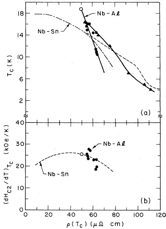
FIG. 2. (a)  $T_c$  vs  $\rho(T_c)$  and (b)  $(dH_{c2}/dT)_{T_c}$  vs  $\rho(T_c)$  for the Nb<sub>3</sub>Al and the Nb<sub>3</sub>Sn systems: (○) bulk Nb<sub>3</sub>Al, (●) Nb-Al this work, (▲) Nb<sub>3</sub>Al radiation damaged, (---) Nb-Sn (Ref. 16), and (—●—) Nb<sub>3</sub>Sn radiation damaged (Refs. 6 and 9).
