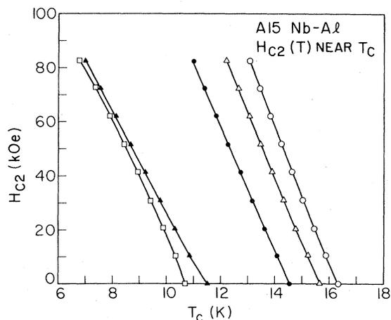
FIG. 1. Representative critical-field data near  $T_c$  of the *A15* Nb-Al films measured. The lines drawn through data points are intended to serve only as a guide to the eye.
