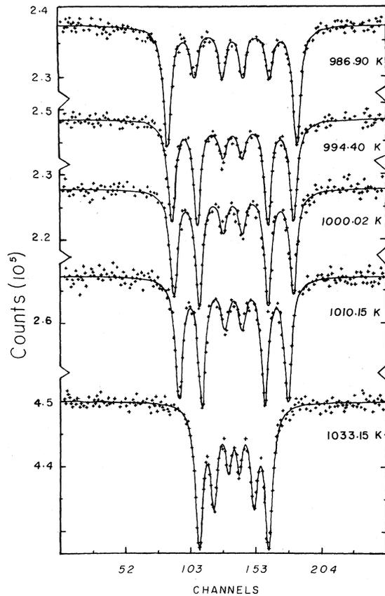
FIG. 14. Variation of line intensity  $I_2$  for an Fe source. ME spectra between 300 and 685 K were similar to  $T = 1000.02$  K. Notice the intensity change of the second line at 986.90 K.
