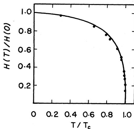
FIG. 2. Reduced hyperfine field  $h(t) = H(T)/H(0)$  as measured by ME in  $\text{Fe}^{57}\text{Fe}$  below  $T_c$ . The solid line is the reduced bulk magnetization as measured by Potter in pure Fe.
