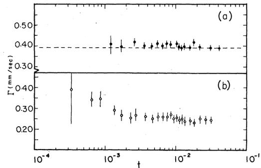
FIG. 6. Variation of the linewidth with reduced temperature below  $T_c$ . (a) The width in the source experiment remains constant and agrees with  $\Gamma = 0.389(3)$  mm/sec calculated from the theory of Margulies and Ehrmann (Refs. 33 and 34) (dashed line). (b) The increase in the width for  $t < 10^{-3}$  in the absorber experiment is due to fluctuations and possible small thermal gradient across the foil (Ref. 27).
