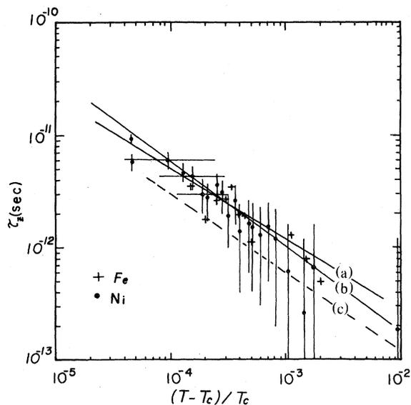
FIG. 10. Autocorrelation times calculated via the theory of Bradford-Marshall. (a)  $\text{Fe}^{57}\text{Fe}$  data (cross points) as obtained in this work; (b) Correlation times (circles) obtained from (ME) in  $\text{Ni}^{57}\text{Fe}$  system (Ref. 27). (c) Dashed line represents the data measured in the  $\text{Ni}^{100}\text{Rh}$  system via PAC (Ref. 26).
