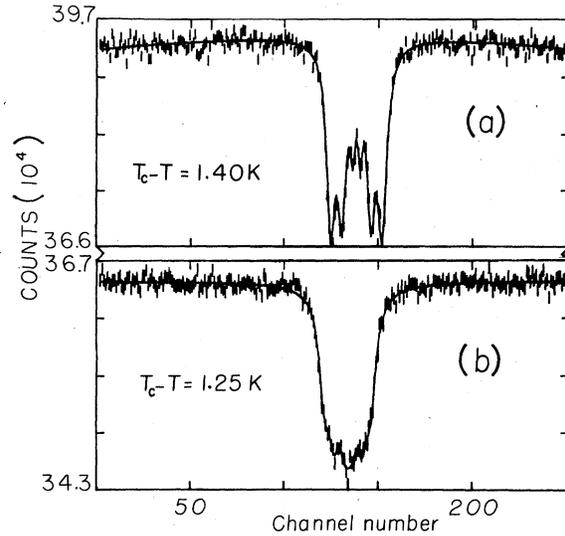
FIG. 1. Close-in Mössbauer spectra in an (a) absorber experiment and (b) source experiment at the same reduced temperature. It can be seen that better resolvable spectra are obtained in the absorber experiment.
