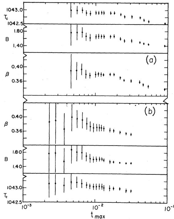
FIG. 3.  $\beta_{\text{eff}}$  measurement in  $\text{Fe}^{57}\text{Fe}$ . The variation of the exponent  $\beta_{\text{eff}}$ , the constant  $B$  and  $T_c$  in  $\text{Fe}^{57}\text{Fe}$  with maximum reduced temperature in both (a) source experiment and (b) absorber experiment. Notice the range of the critical region where  $\beta_{\text{eff}}$ ,  $B$ , and  $T_c$  remain constant.
