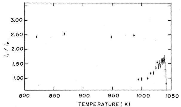
FIG. 15. Behavior of  $I_1/I_2$  as a function of temperature. For  $800 \text{ K} < T < 986.9 \text{ K}$  the value  $I_1/I_2$  remained 2.5 and dropped to 1 outside this range. Notice the abrupt change at about 990 K.  $I_1/I_2 = 1.5$  corresponds to random domain alignment.  $I_1/I_2 \rightarrow \infty$  corresponds to domain alignment in a direction parallel to gamma ray.  $I_1/I_2 = \frac{3}{4}$  corresponds to domain alignment in a direction perpendicular to the gamma ray.
