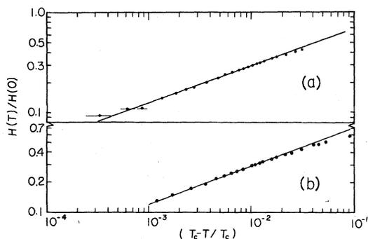
FIG. 5. Logarithmic plot of the reduced hyperfine field for (a) absorber and (b) source experiment. The breakdown of the power law at  $t = 2 \times 10^{-2}$  can be seen in both cases.
