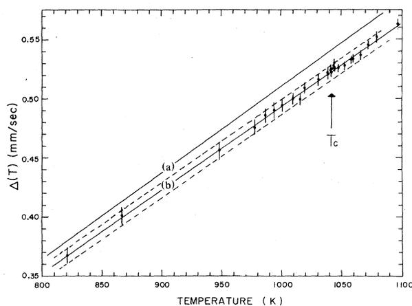
FIG. 12. Energy shift in  $\text{Fe}^{57}\text{Fe}$  in the neighborhood of  $T_c$ . Curve (a) indicates the theoretical SOD calculated via the first term of Eq. (27). Curve (b) illustrates a linear fit to total shift measured. The dashed lines show the systematic error.
