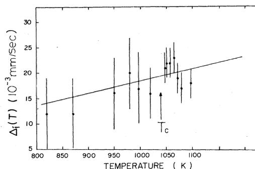
FIG. 13. Isomer shift variation with temperature as obtained by subtraction of the second-order Doppler shift (SOD) from the total shift measured.
