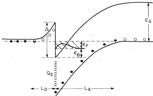
FIG. 1. Diagram of the heterojunction at equilibrium in zero magnetic field.
