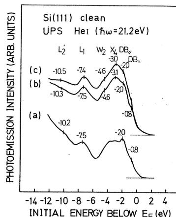
FIG. 1. UPS spectra of three Si(111) surfaces thermally cleaned with different surface preparation techniques: (a) after flash cleaning the surface to remove the surface native oxide, (b) after annealing around 900 K, (c) after high-temperature annealing above 1200 K and subsequently quenching to room temperature.
