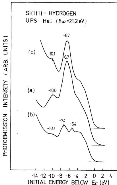
FIG. 2. UPS spectra after saturation with atomic hydrogen chemisorption for the three different clean Si(111) surfaces (see text), resulting in the monohydride (b) and the trihydride (a) and (c).
