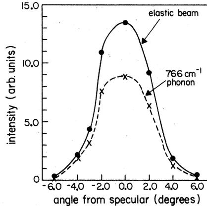
FIG. 4. Intensity versus angle from specular beam direction for 14-eV electrons on TiO<sub>2</sub>(100),  $T = 309$  K. The phonon loss intensity is multiplied by 2.
