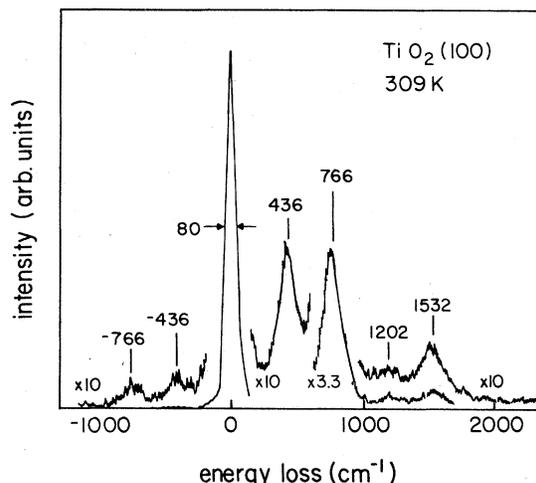
FIG. 2. Energy-loss spectrum of 14-eV electrons in specular reflection. Angle of incidence is 50 degrees.
