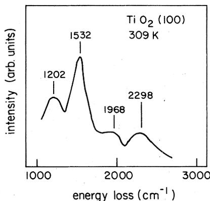
FIG. 3. Energy-loss spectrum as in Fig. 2 showing higher-energy region. Vertical lines indicate the predicted positions of multiphonon excitations of  $\nu_1, \nu_2$  as in Table I.
