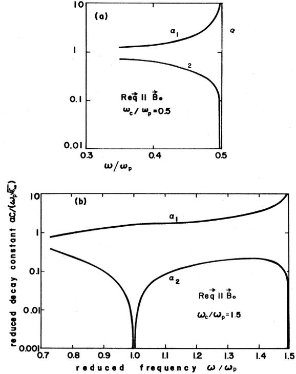
FIG. 2. The decay constants  $\alpha_1$  and  $\alpha_2$  of the interface modes shown in Fig. 1 for two values of the parameter  $\omega_c/\omega_p$ : (a) 0.5, (b) 1.5. Only the frequency region of bona fide modes is shown. Note the logarithmic scale.
