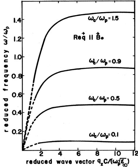
FIG. 1. Dispersion relations of magnetoplasma modes at the interface between a highly doped semiconductor and a metallic screen in the Faraday geometry. For every value of the static magnetic field  $B_0$  there is one mode, and it terminates at the cyclotron frequency  $\omega_c$ . Continuous lines indicate a bona fide interface mode whose decay constants are both real and positive. Broken lines indicate a generalized interface mode whose decay constants are complex conjugates.
